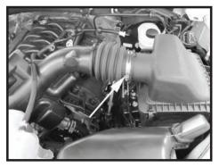
Step 4 Loosen the clamp at the air filter housing and then remove the intake tube from the vehicle.
