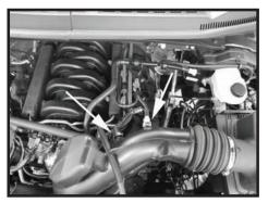
Step 2 Disconnect the PCV fresh air hose and vent hose from the intake tube.
