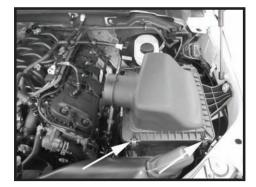
Step 5 Unclip the two hold down clips on the air filter lid, lift the lid then slide it forward to clear the locking tabs. Remove the air filter lid and air filter.
