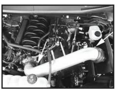
Step 10 Install the Spectre Performance intake tube into the flex coupler on the heat shield then into the coupler on the throttle body. Fasten securely in place.
