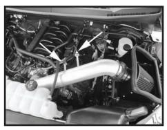
Step 11 Reconnect the PCV hose and vent hose into the intake tube.
