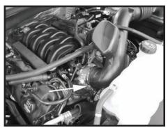
Step 3 Loosen the clamp on the tube going to the throttle body.
