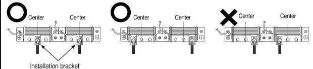
● When installing and using the "RF18" unit, make sure to install 2 Installation brackets (Item ②) at 2 positions on each lamp.
