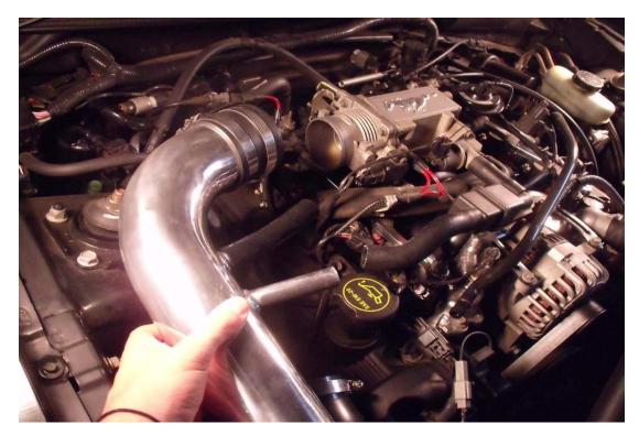
4. Remove the electrical connection clip by pinching the bottom of the clip and pulling the connector straight off.
