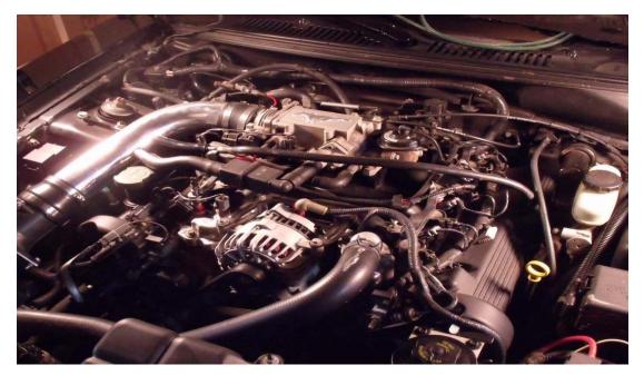
2. Next remove the upper intake pipe using a Flat Head Screwdriver to loosen the pipe clamps. This may vary depending on the set up of your intake.
