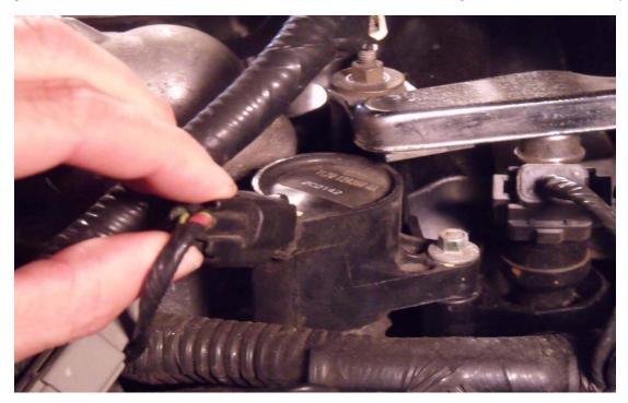
6. Next, pop the coil from over the spark plug making sure to clear the fuel rail. Then, pull the coil straight out from the engine.
