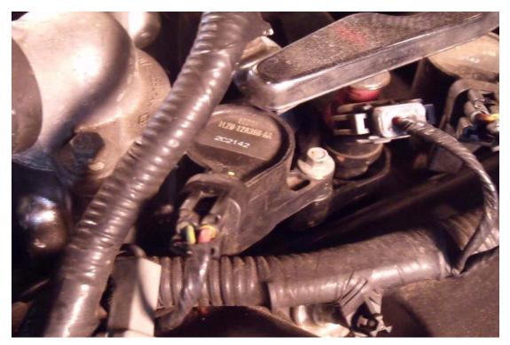
5. Using the small socket wrench, or a socket driver, with a 7mm socket, remove the single bolt that holds the coil in place.
