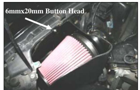
9. Install the Airaid Premium Filter (#1) onto the velocity stack inside of the CAD as shown and tighten the clamp. Next install the CAD assembly into the vehicle aligning the grommet posts into the factory grommets in the inner fender. Now secure the CAD to the inner fender well using the 6mmx20mm button head bolt (#9), and flat washer (#11).
