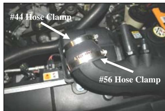
8. Install the reducer coupler (#4) onto the throttlebody end of the Airaid Intake Tube using the #56 hose clamp (#14) on the tube end, and the #44 hose clamp (#13) on the small end. Tighten *only* the large #56 clamp at this time.
