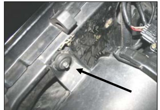
3. Remove the bolt that holds the factory air filter canister to the inner fender. Next remove the factory air intake tube from the throttlebody, and then the MAF housing. Now with a twisting motion remove the factory air filter canister from the vehicle.
