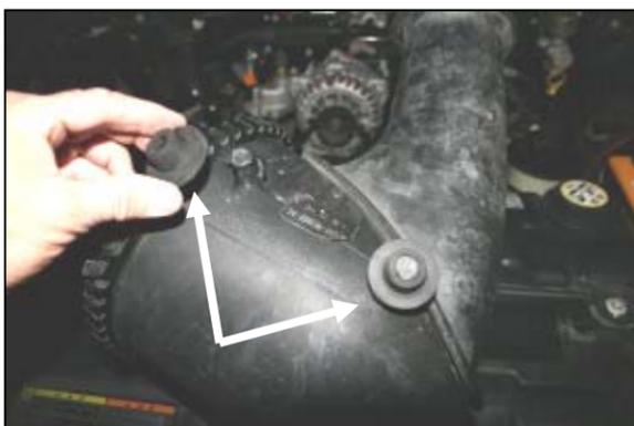
4. Remove the two factory grommets from the bottom of the factory air filter canister and reinstall them into the holes in the inner fender.
