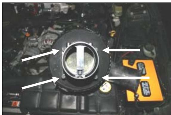
5. Remove the four bolts that hold the MAF housing to the factory air filter canister. The bolts will not be reused, but the MAF housing will be used in the next step.
