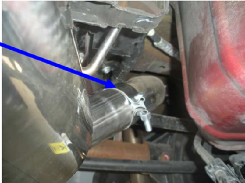
New band clamp attach Bassani muffler to over- axle pipes
