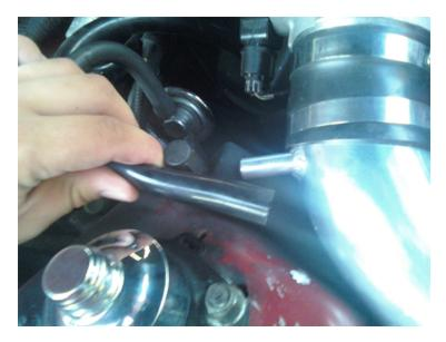
3. Disconnect the Throttle Position Sensor, located on the left side of the throttle body, by removing the two (2) screws on the top and bottom of the sensor.
