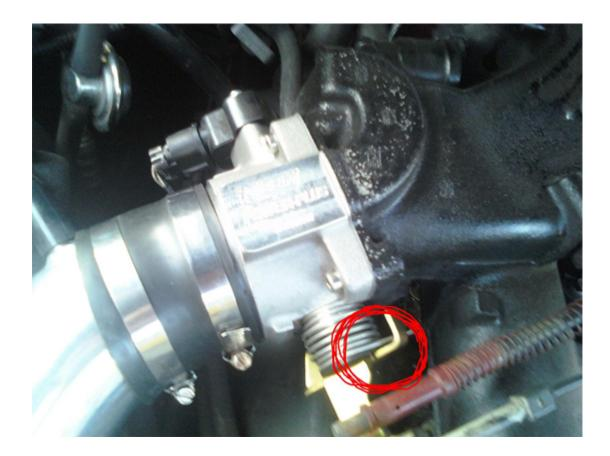
17. If your car does not start properly, after idling until the engine is at its normal operating temperature, you will have to adjust the idle screw located under the red circle in the picture above. You may need to open the throttle body by pushing the screw against the throttle body to open the throttle butterfly more by using the 3mm Allen wrench. This should fix any start up problems you may encounter.
