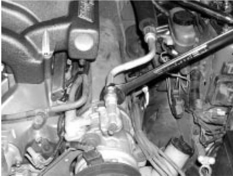
9. Re-establish all upper manifold connections that you disconnected in step 5.
