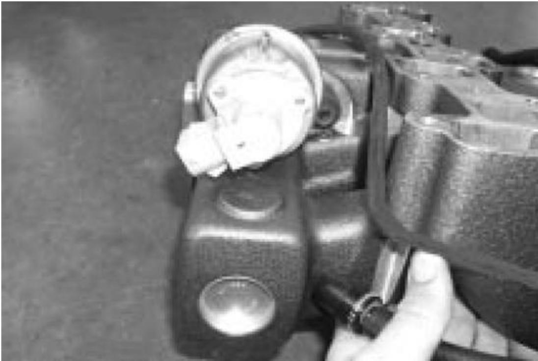
5. Transfer the EGR valve, throttle body\*, and throttle cable bracket to the BBK upper \*(5002 customers will install the supplied throttle body and transfer the IAC valve) using the 5/16-18 x 5/8 bolts and the supplied gaskets for the throttle body, and the stock bolts for the bracket. (If your vehicle has cruise control install the supplied spacer between the upper manifold and throttle cable bracket using the two M-8 x 1.25 x 30 SS-BHCS. The spacer only installs one way).
