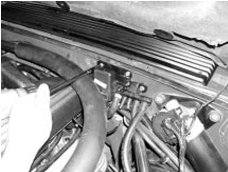
11. Using the supplied gasket and the final 6 10-32 SS-BHCS attach the plenum cover to the upper manifold.
