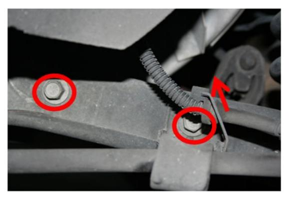
4. I did this on both sides of the vehicle and moved the sway out of the way. If you were planning on replacing your sway bar now would be a good time to do so.
