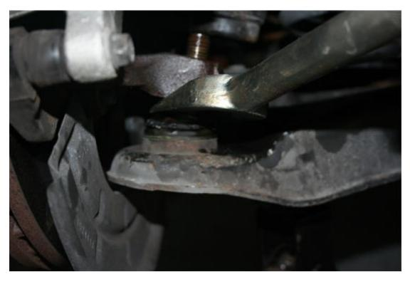
Now with these items removed and separated lower the jack to release tension off of the spring. Then use your foot for a little extra clearance and remove the stock spring. 16.
