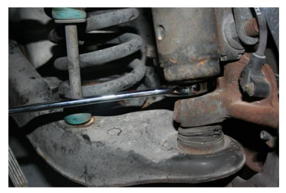
I replaced the ball joints also at this time, so I used a pickle fork to separate the ball joint from the spindle. However you may use you mallet again to break this joint. The use of a pickle fork does require the replace of the ball 15. joints
