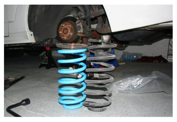
8. Insert the new spring and ensure that where the spring is cut on the bottom is facing toward the driver's side of the vehicle. Jack the control arm back up into place and bolt it back together. Repeat for the other side with the same instructions and then reinstall the sway bar and tires.
