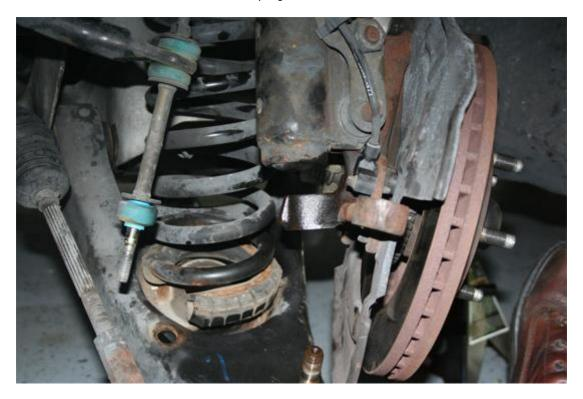
17. Place the isolators on the new spring and install it in the control arm.
