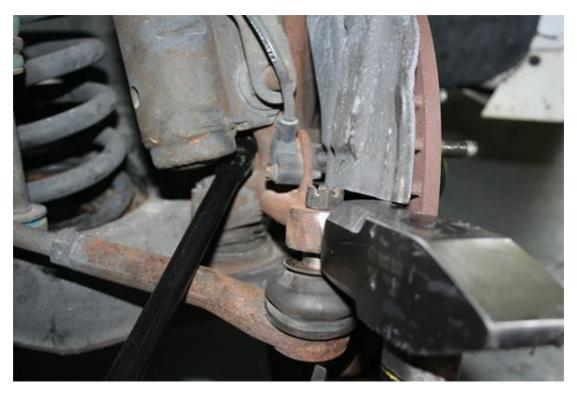
14. Next take the jack and use it to apply pressure to the spring by jacking up the control arm, then remove the nut securing the ball joint to the spindle with a 24mm wrench.
