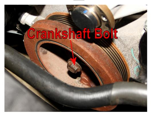
17. Then thread the bolt all the way down by hand.
