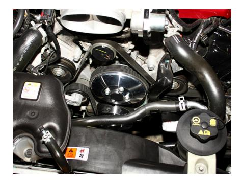
32. Your pulleys are installed, and you're ready to go. Enjoy your newfound power, and especially the fact that the underdrive pulleys have freed up the engine some in the lower RPM range!
