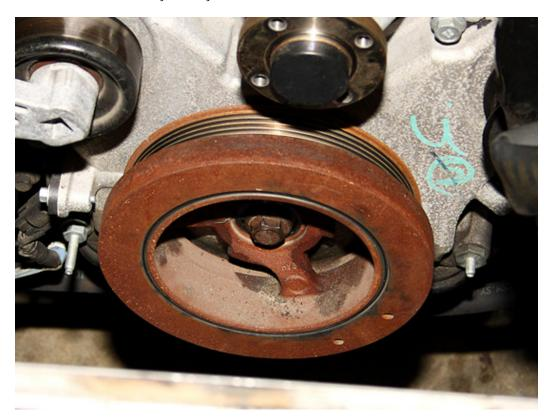
18. The balancer for the 4.6 does not use the threaded holes that are typically used on Fords. Instead the offer three balancer perches for a three-jaw puller, similar to older Chrysler balancers.
