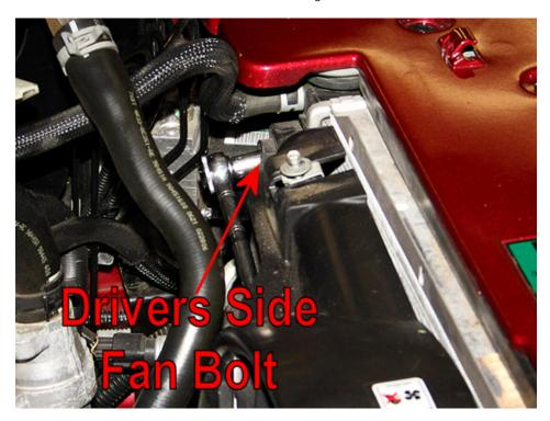
15. With the two bolts removed, the fan assembly will lift straight up and out. You will have to work it past a few hoses and harnesses. I found it easiest to shift it to the driver's side of the engine bay, clear the upper coolant hose with the fan assembly's mounting tab, then work the other side of the fan assembly up and out. With the fan out, you can see the various mounting locations, and the wiring plug.
