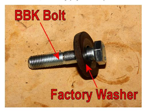
23. Set the balancer onto the crankshaft, ensuring that the keyway opening matches the spline on the crankshaft. Then thread the BBK bolt into the crankshaft. Use the bolt to pull the balancer onto the shaft. The BBK bolt will stop after a few turns, do not overturn it. The BBK bolt is only intended to pull the dampener on enough so that the factory bolt will fit. When the BBK bolt stops, remove it and the factory washer.
