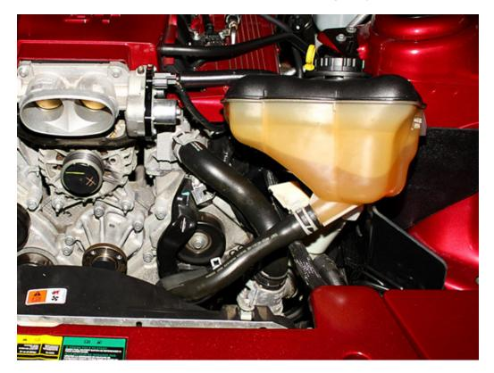
12. The wiring plug for the fan is a little tricky and hard to access, due to it being directly under a wiring harness. It can be found under the area the coolant tank sat. Press in on the plug tab, and then pull it away from the fan.
