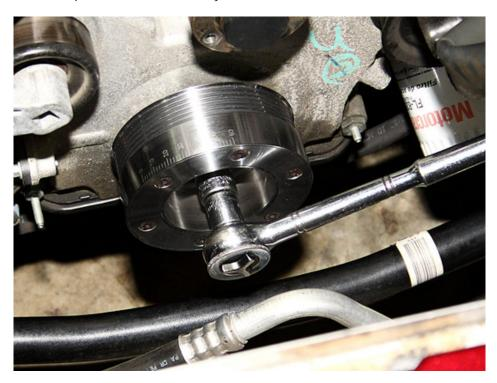
24. Then, place the factory bolt back in the factory washer, and reuse the factory bolt to pull the dampener fully onto the crankshaft. There will be only a small gap between the back of the damper and the engine block. You will feel the bolt start to tighten up, and the engine's crankshaft start to rotate when this occurs.
