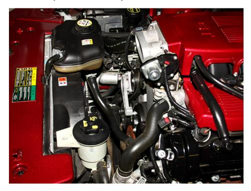
3. Next, loosen the bolts holding the water pump, but do not remove them yet. The belt will help prevent the pulley from turning, but you'll probably have to use your hand to help hold it as well. These bolts need a 10mm socket.
