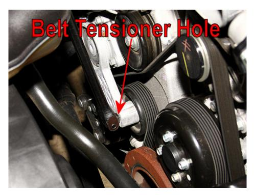
7. Lift the belt off of the alternator pulley. You can go ahead and remove the water pump pulley bolts, and water pump pulley at this time.
