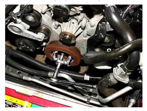
20. With the balancer now removed, clean the crankshaft of any grime and leftover sealant.
