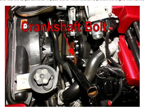
5. Once loosened, the bolt should turn out easily by hand. Make sure you remove the factory washer as well. It will probably still be on the balancer.
