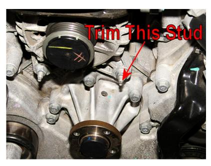
28. I used a Dremel with a cutting wheel, and performed this task in a matter of seconds. Cut the excess non-threaded portion of the stud off as shown. It's a good idea to cover the alternator, throttle body, and water pump weep hole from stray metal dust. The weep hole can be seen in the picture below, just to the left of the stud you're cutting.
