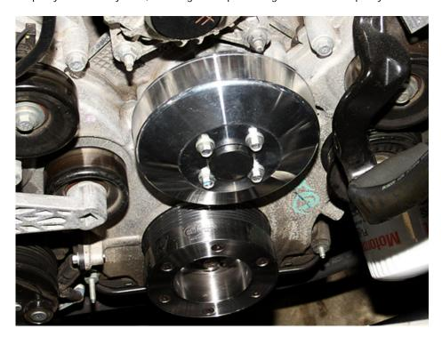
30. Place the belt back on the accessories, using BBK's diagram below for proper routing. You'll need to use a ½ inch socket wrench on the belt tensioner to get the belt into place. Once the belt is in place, check and retighten the water pump pulley bolts.
