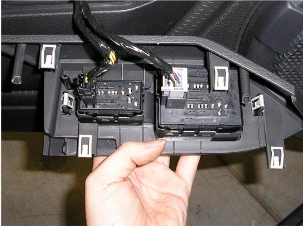
5. Remove the door lock bezel by wrapping your small jeweler's flathead in a shop towel and prying upwards.
