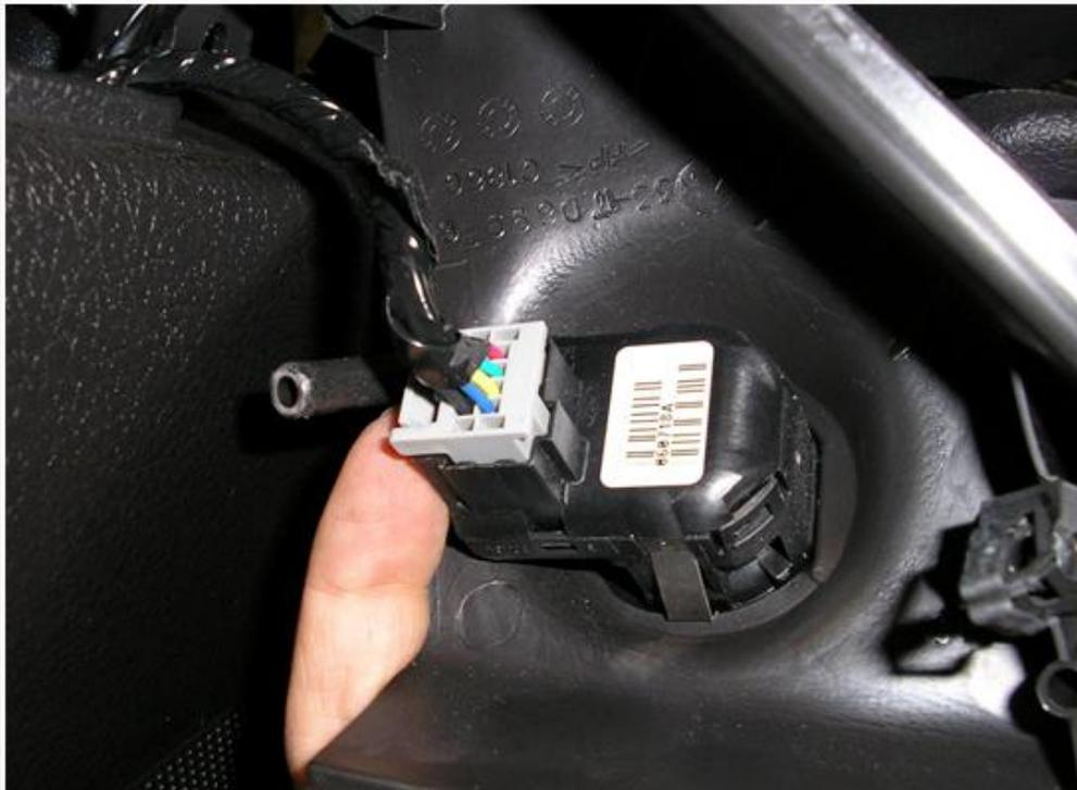
10. Remove the interior panel by lifting up on the handle. Remove any electrical connections.
