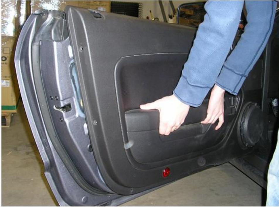
11. In order to remove the door release cable, you will need to remove the door handle assembly. To do this, use a small flathead screwdriver wrapped in a shop towel to pry away the faceplate and/or push from the back of the assembly. There are two clips on the bottom. You will need to use a significant amount of force.
