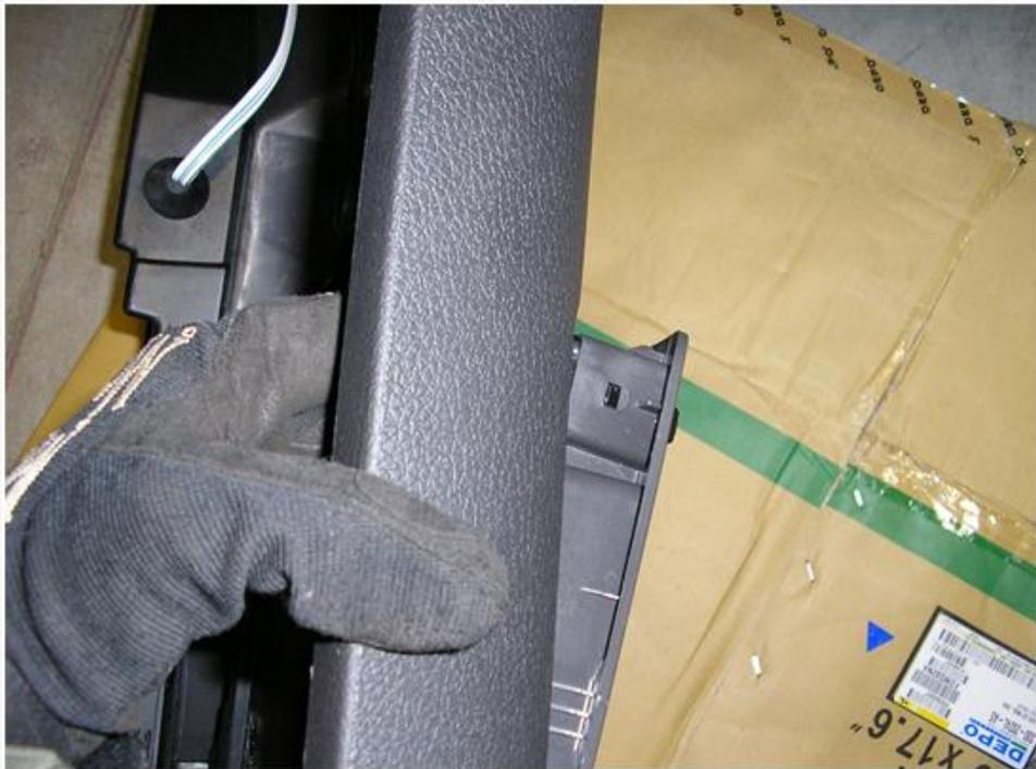
12. Rotate the door handle assembly and slide it out the back of the door.
