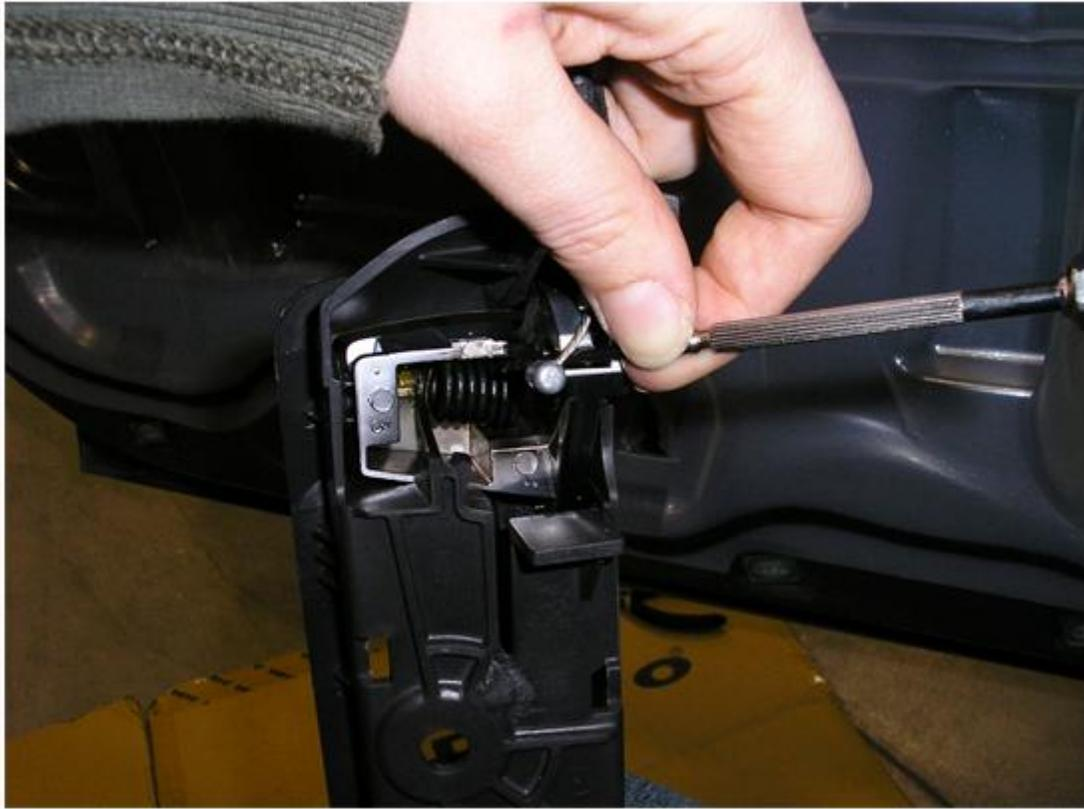
14. Remove the stock handle from the cup. The easiest way to do this is to first remove the spring with a jeweler's screwdriver. Use the screwdriver to pry out the center of the spring then lift its long "leg" out of the recess where it sits. Use caution and wear eye protection as the spring will jump abruptly out of the cup once released. Be very careful not to damage the spring as it will be reused.
