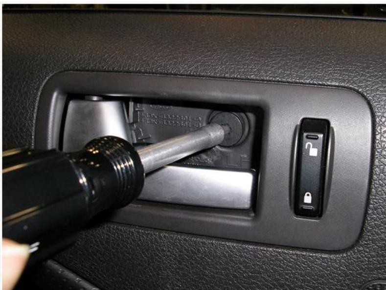
2. Remove the cover from the door pull/armrest area. You may need to use a small jeweler's flathead to pry it forward and away from the main door panel to release it. Remove the T30 Torx screw from behind it.
