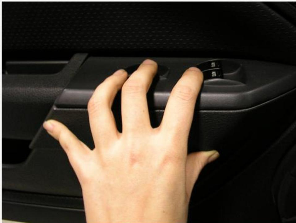
4. Remove the 2 plugs from the switches.
