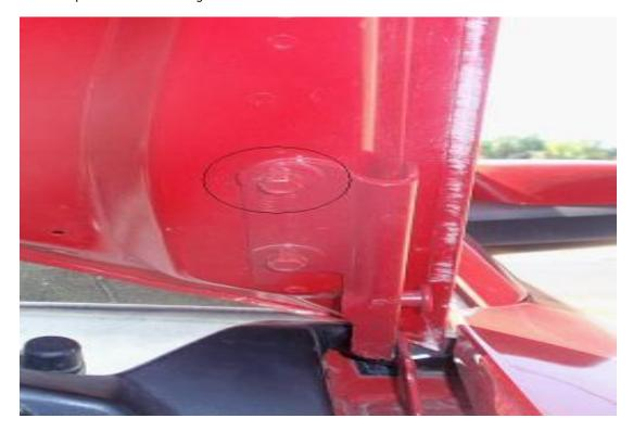
5. Locate the large bracket marked D-U. Now loosen the bottom bolt on the hood hinge just enough to slide the larger bracket between the hinge and the bolt as shown. DO NOT REMOVE BOTTOM BOLT. Tighten bottom bolt first and than re-install top bolt to secure bracket. ( Note: Align the top bolt holes before tightening the bottom bolt.)
