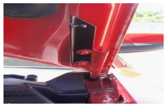
6. Once the bracket is firmly secured to the hood hinge, install the gas strut by popping the ends over the ball mounts on the bracket as shown. (Note: If you need to remove gas strut after it is installed use the flat-head screwdriver to pop out the metal brace at the ends of the gas struts. Make sure to put the brace back on the strut before installing it again.)
