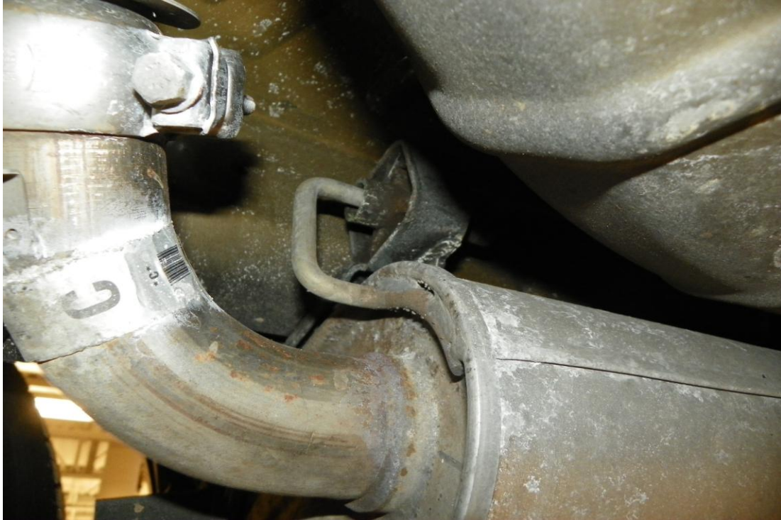
Rubber hangers which hold the muffler towards the front of the car
