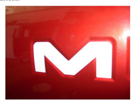
7. After a few seconds, take your fingers and run them over the letter squeezing out all of the water. Make sure there are no pockets of water or air bubbles behind the letters and if there are, simply work the bubble to the edge of the letter.
