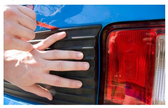
6. Since the adhesive is pressure sensitive at this point I popped the trunk open to make sure I had applied enough pressure around the entire perimeter of the panel. It can take up to 24 hours for the tape to fully cure.
