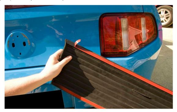
3. Align the decklid panel on the rear of the car so that there is an even amount of body on each side of panel. For me there was less than an eighth of an inch remaining and the fit was great.
