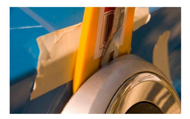
6. The emblem will make its way off and you'll be left with the rear of the car most likely having two plastic retainers as I highlighted on the above photo. I removed those and pushed them onto the emblem.
