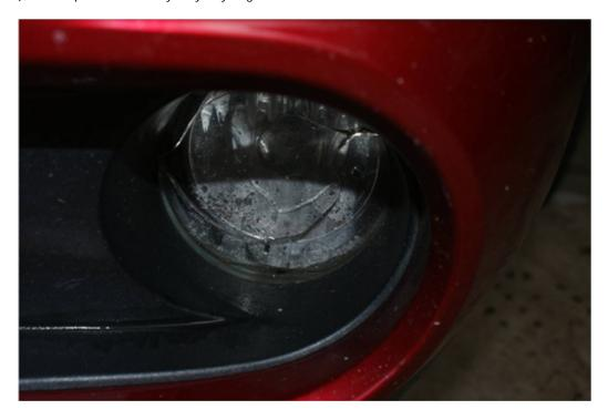
3. It is best to replace one fog light at a time so that you have the other to reference incase you accidently install the light the wrong way or other mistakes occur during the install. Remove the clip from the back of one of the lights.
