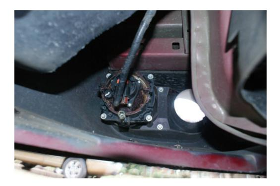
4. Remove the clip from the back of the fog light. Next you need to remove the four 7 mm bolts from the old fog light bracket. Make sure, however, that you do not remove the two 7 mm bolts that are holding in the black trim piece in front of the fog light bracket.
