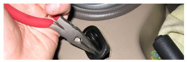
3. Pull the selector through the console, to where the coin holder was. You will need to remove the knob on the selector, by simply pulling upwards.
