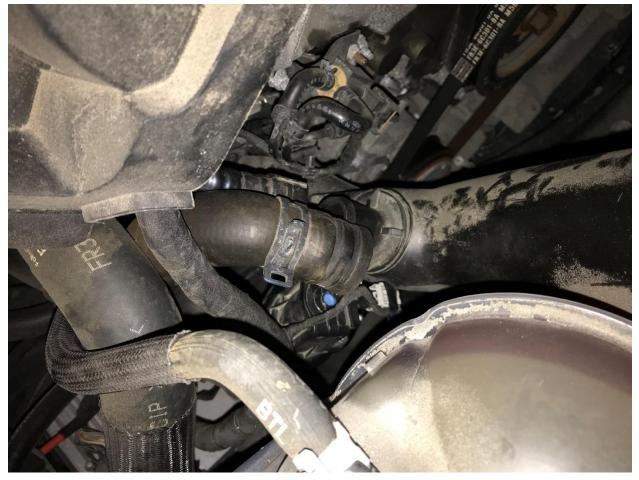
**Step 9:** Place new tube into the car and slide over turbo inlet coupler first followed by the airbox side. Reattach PCV and turbo bypass lines and tighten clamps.
