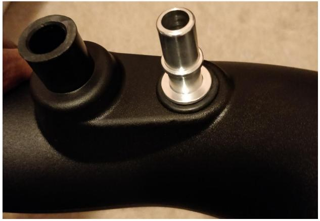
**Step 3:** Insert the rubber grommet followed by the aluminum fitting into the intake tube.
