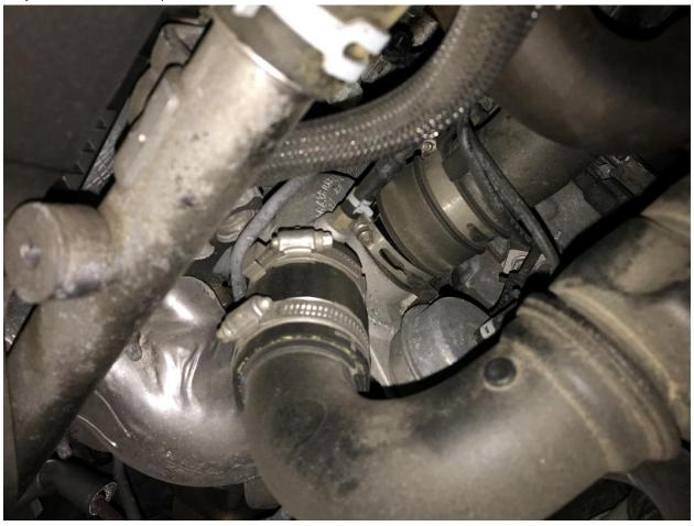
**Step 7:** Loosen the clamp on the outlet side of the stock intake tube.
