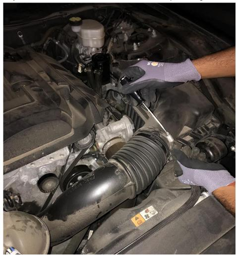
**Step 6:** Disconnect the inlet side of the old intake tube by loosening and twisting the clamp.
