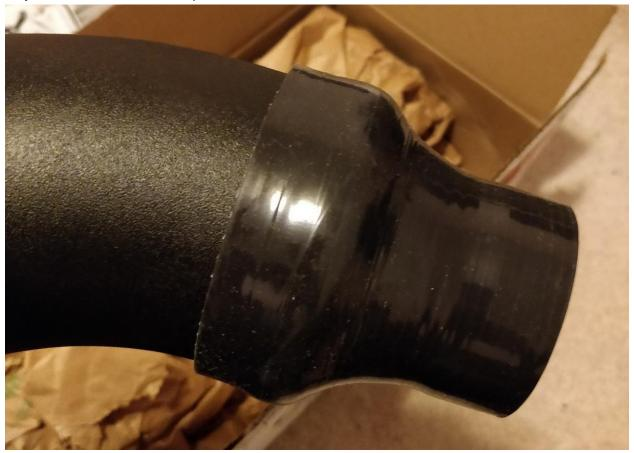
**Step 2:** Use clamp #56 on the smaller end and clamp #68 on the large end to secure the couplers. Tighten with a flathead screwdriver.
