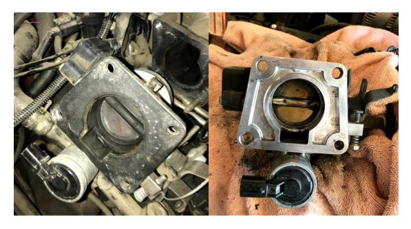
7. Remove the 3 studs from the manifold. To remove these, take 2 nuts that were removed from step 3 and put them on the same stud as shown below. Tighten the nuts against each other and then begin to remove the nut closest to the manifold. If this is done correctly, the stud will back out.
