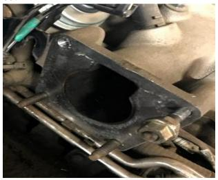
8. Now install the Aluminum spacer and the 2 gaskets. Make sure the side of the spacer that is stamped "T.B. SIDE" is facing the throttle body. (if you install this reversed the spacer will not operate correctly)
