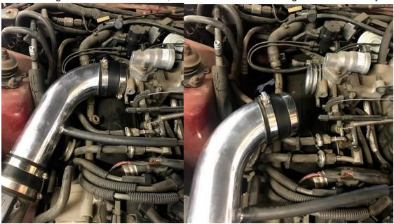
3. Using a 10mm socket and extension, remove the 3 nuts and 1 bolt (4 total) that hold the throttle body to the manifold
