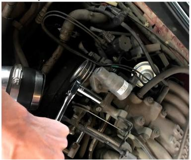
4. Using a 10mm socket, remove the 2 bolts from the throttle linkage bracket.
