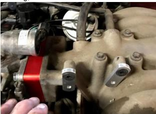
10. Tighten down the linkage plates so that they are horizontal and facing the throttle body. Now take the 2 5/16-18 bolts and washers and use them to install the throttle linkage bracket. NOTE: beware, when tightening the bracket, the linkages will want to rotate.
