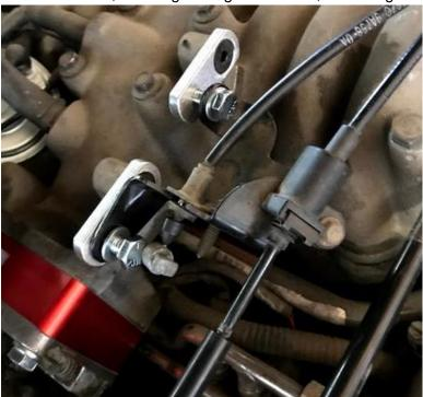
11. Inspect the throttle body area and ensure the all cables and springs are still connected to the correct areas.
