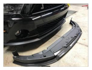
2. Remove OE spoiler from vehicle by removing 12 bolts and 4 screws underneath the OE spoiler
