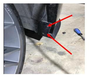
4. Install New Spoiler by first clipping the tabs on the spoiler to underside of front bumper
