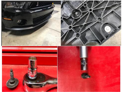
3. Remove 4 bolts (2 each side from Wheel well)
