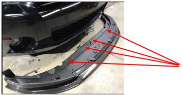
8. Install 2 bolt/screws (2 in each side of wheel well (Note: holes must be drilled in new spoiler as they are not drilled from the Factory)
