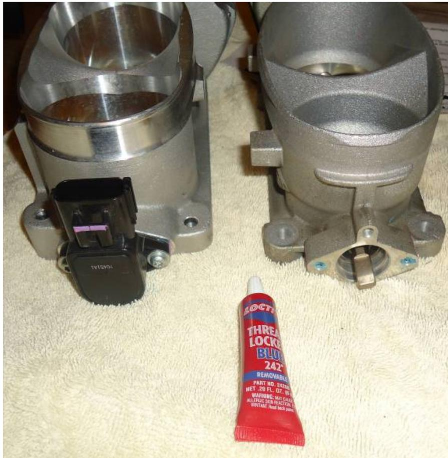
12. Use your T20 Torx bit to remove the bolts holding the motor housing to the old TB. It is not necessary to remove the 2 bolts securing the motor housing; see the picture below.
