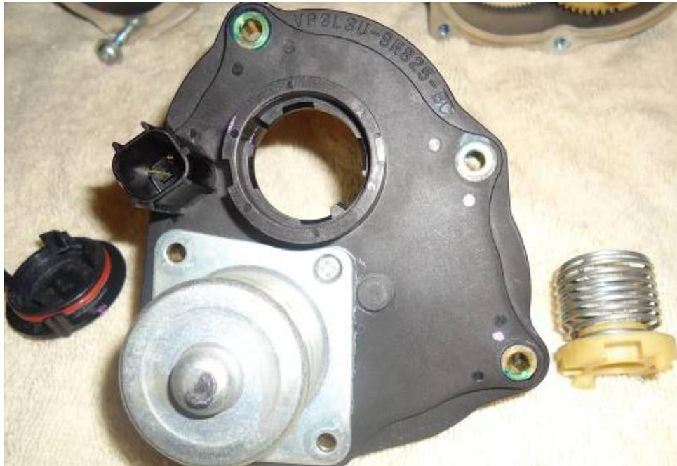
14. Place the spring into the new TB. Insert the tip of the spring into the hole in the top gear.
