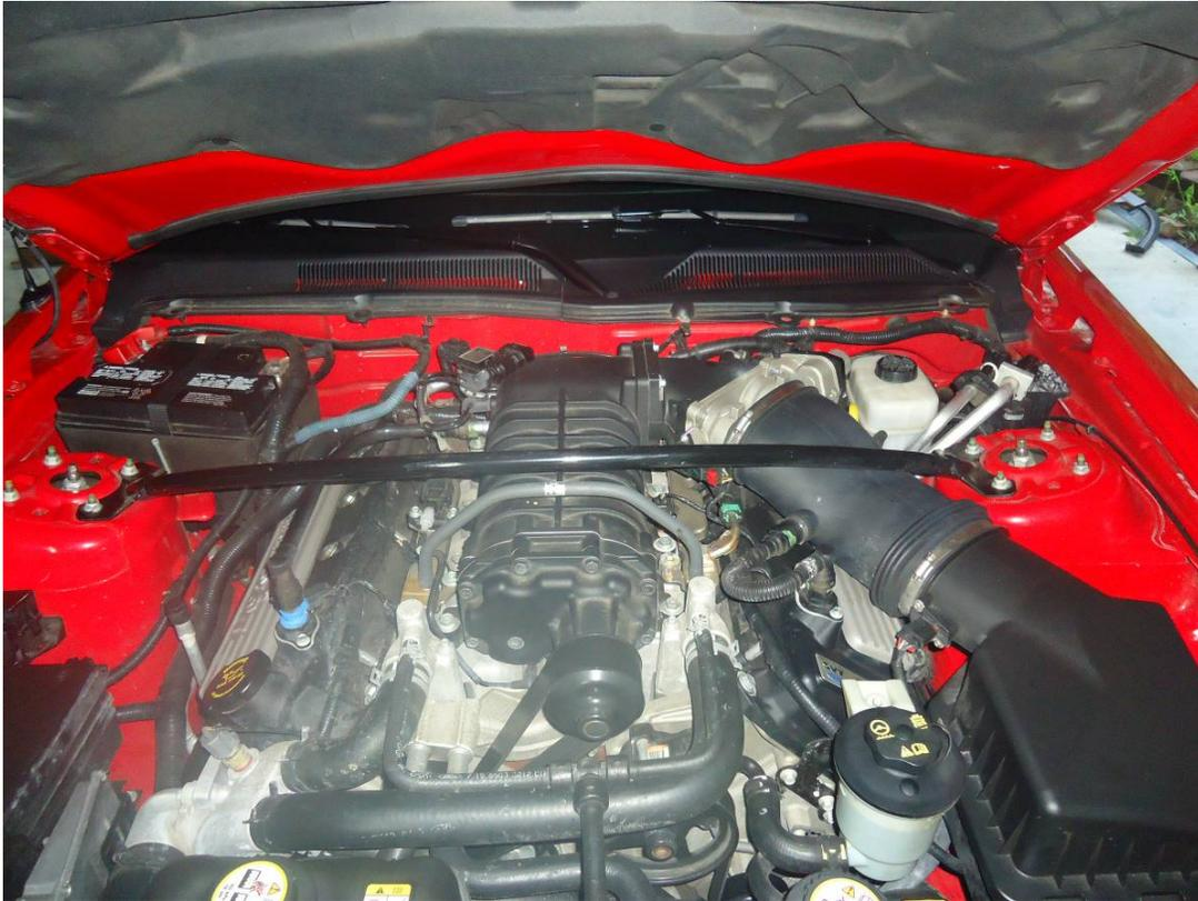
4. If you have an aftermarket CAI, remove it from your fender. If you have the stock airbox, use the 13/32" socket to remove the bolt holding it to your fender. On the MAF Sensor connector, pull out the red tab and remove the connector.
