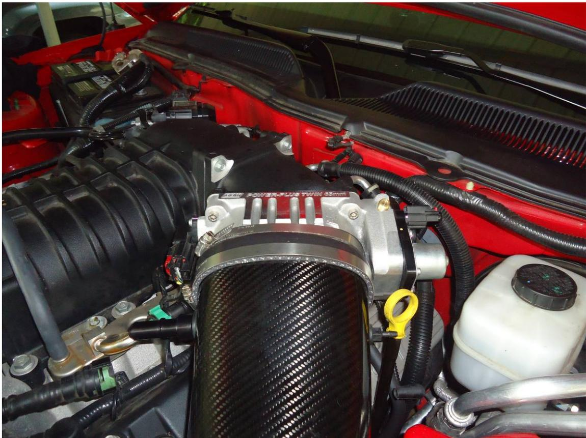
21. Attach the MAF connector to the inlet tube and press in the red tab to lock it in place. If you installed an aftermarket CAI, you will need to transfer the MAF Sensor from your OEM tube to your new tube.
