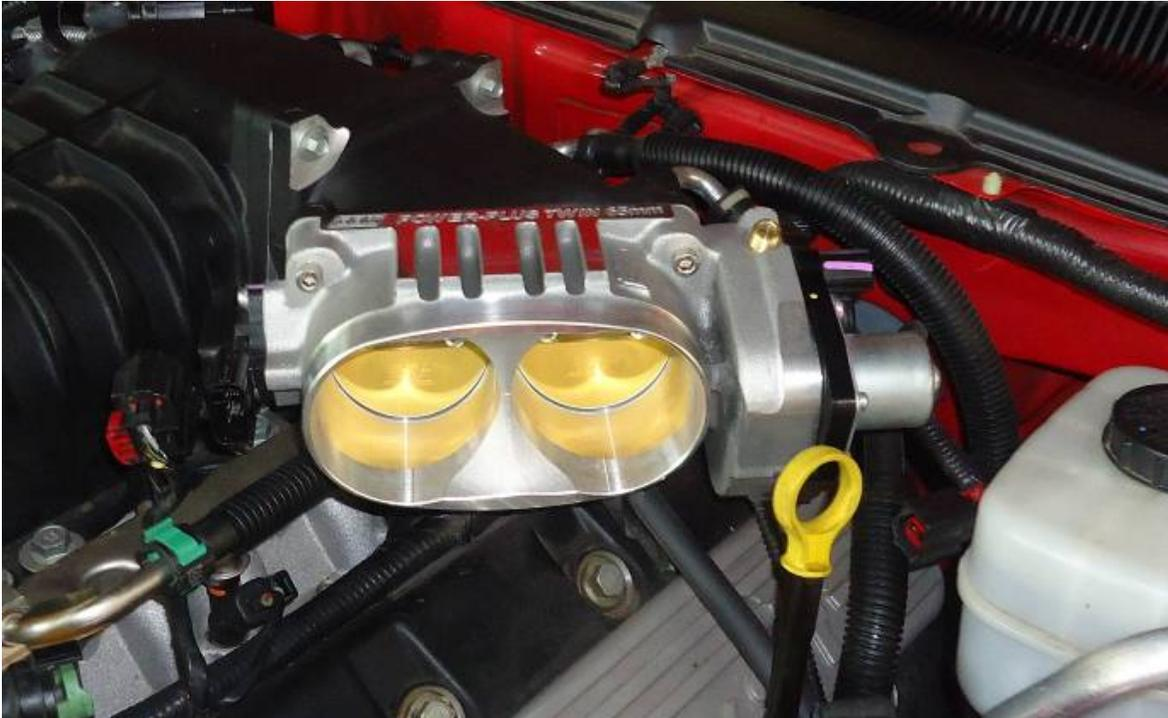
19. Reinstall the two connectors to the TB. Press in the red tabs to lock them in place.
