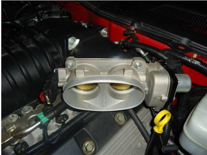
7. On the left connector of the throttle body (TPS), pull the red tab out on. Disconnect from the throttle body. On the right connector (Motor Housing), do the same.
