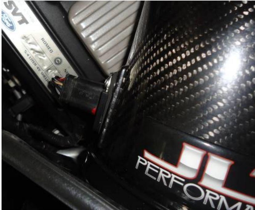
22. Slide the PCV tube onto your inlet tube. The green locking connector will snap into place. Slide the vacuum hose on and make sure it is secure.
