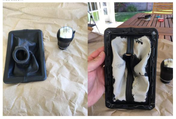
3. Once the old boot is removed begin to remove some of the left over adhesive that may be stuck on both sides of the frame. Use your flat head screw driver to scratch left over leather. This will take some elbow grease and patience to fully remove the gunk left behind.
