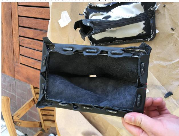
2. Spread on a small dab of contact cement or Crazy Glue on the bottom side of each corner of the frame and folding the leather tightly. I used large binder clips to hold the leather together while drying. Re use the O-ring that secured your old boot and re install it using super glue.
