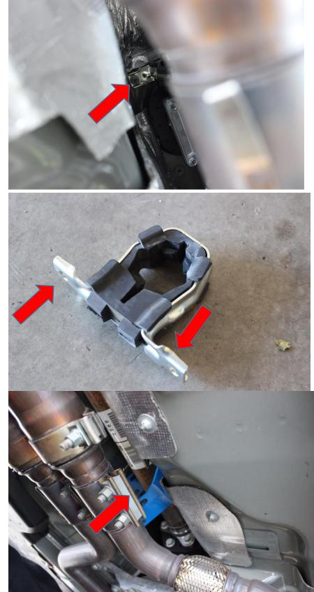
Loosen 3 15mm bolts on transmission just enough to fit lower bracket on
