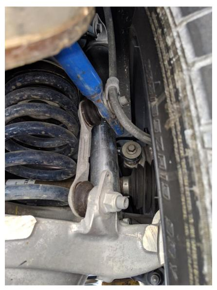
Now that you removed the old links start by installing the new BMR link (from the back side just like the one removed)
