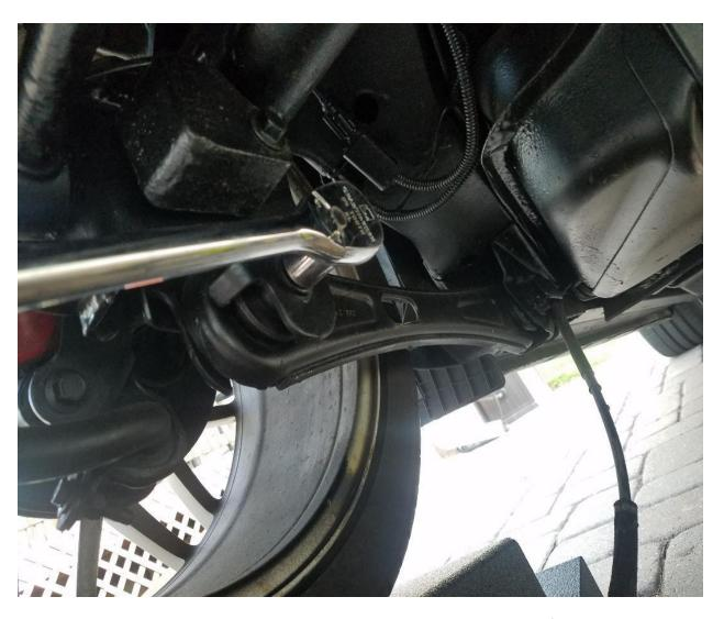
4. Remove the rearmost lower control bolt with your 18mm socket, the nut for this bolt has a built in flange that stops it from spinning so there is no need to hold it.
