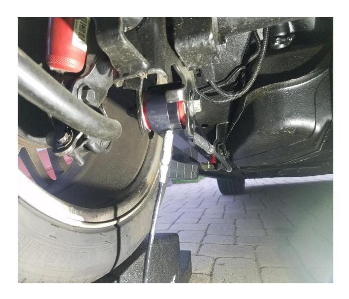
9. Take your grease gun and connect it to both the fittings on each arm and give each fitting 2-3 full pumps of synthetic grease. Repeat these same steps for the passenger side rear control arm. Your install is now complete, take the car for a drive and make sure you don't hear any weird noises. Since these bushings are much stiffer then stock you will have a slight increase in NVH but much better traction. Enjoy your new BMR Billet Rear Lower Control Arms
