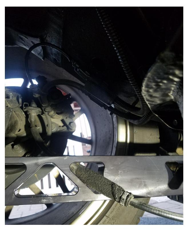
8. Feed your parking brake cable through the middle rear slot in the BMR arm (you can also just zip tie it to the side of the arm if you prefer but I prefer this cleaner look like stock). Slide the cable retaining clip back into its slot and reconnect the parking brake cable to the brake caliper.
