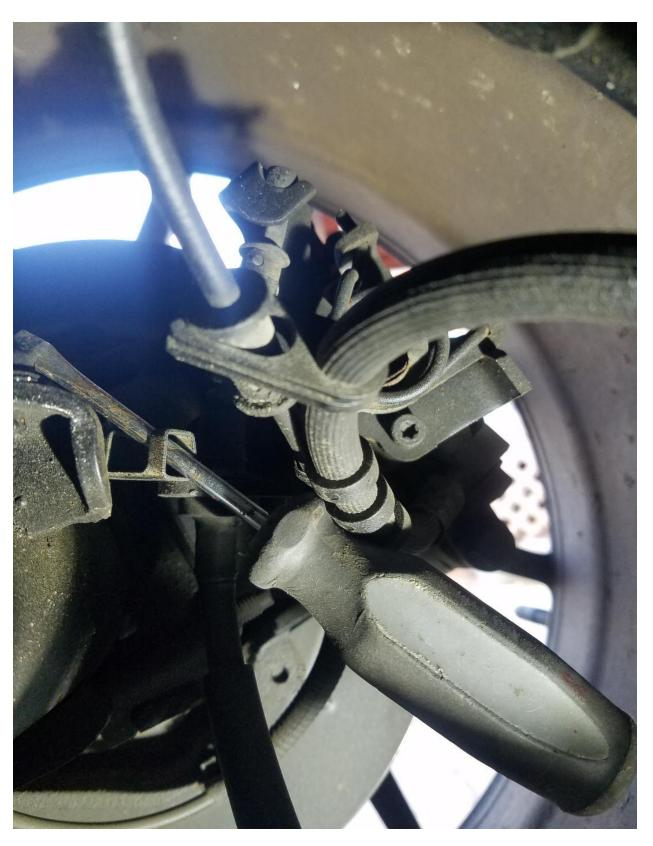
2. Take a flat head screwdriver and remove the parking brake cable retaining clip by simply sliding it off.
