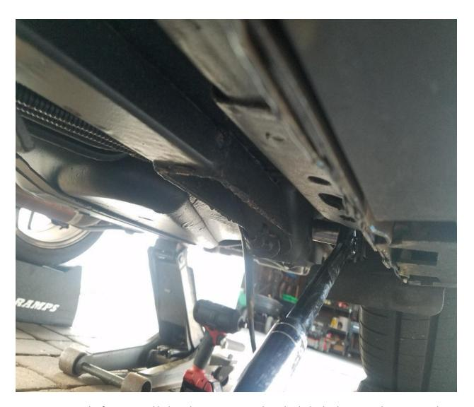
5. Remove the front control bolt with your 18mm socket; this bolt also has a nut that stays in place on the body so no need to hold it. Once the bolt is removed the control arm will fall out so hold it while you are removing the bolt.
