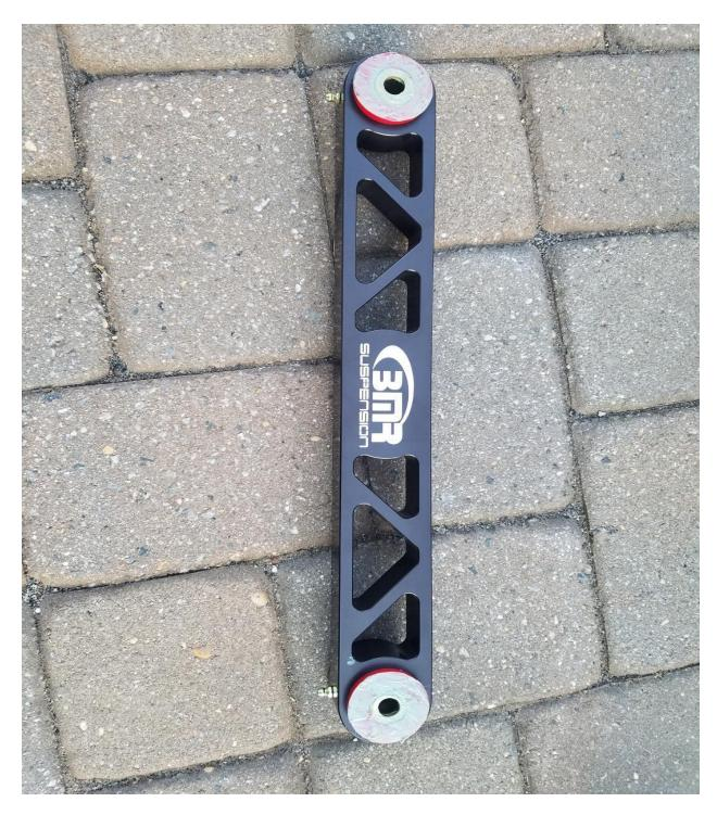
6. Prepare your new BMR billet control arms by applying a small amount of grease to the 4 outer bushings as shown.
