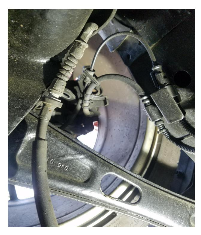
3. Slide the parking brake cable out of the caliper then through the control arm and secure it away from the control arm.
