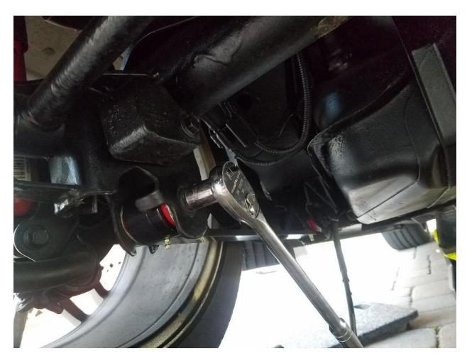
7. Install your new BRM billet arm with the smaller side bushing forward, BMR logo facing outward and grease fitting facing down. Reinstall the 2 18mm bolts removed in the previous steps and torque them to 130 ft lbs each, the suspension should be loaded when doing this so ramps are ideal.
