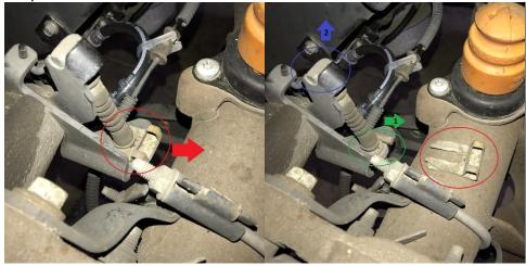
5. Remove the factory front 18mm control arm bolt (the nut may stay in place or fall out of its bracket) and remove the control arm from the front mount.
