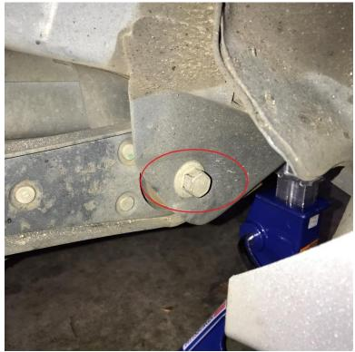
6. Remove the factory rear 18mm control arm bolt and remove the control arm from the rear mount.
