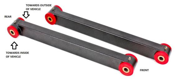
15. Install control arm into desired hole in relocation bracket with hardware #9 and #2. This may require a pry bar, ratchet strap, rubber mallet, or other creative ways to accomplish. Removing weight on axle by lowering car
