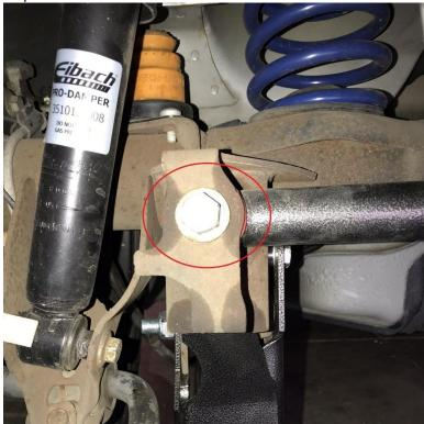
21. Install the driver's side relocation bracket by reinstalling axle weight (if equipped). If it was not equipped use, hardware #8 (19mm) and #5 to attach relocation bracket to axle. The spacer installs in-between the axle and new bracket. Do not tighten.
