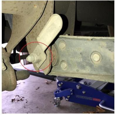
7. If equipped on vehicle, remove the axle weight with a 15mm socket and wrench. If not move to next step.
