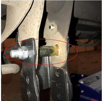
10. Install #7, #4, and #2 in the top backside mount. Place bolt through washer and thread nut on bolt. Place 22mm wrench through bracket on nut. Torque 22mm bolt to 129 lbs/ft.
