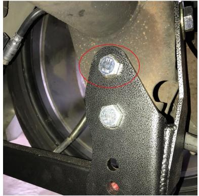
9. Install hardware #1, #2, and #3 for the lower bracket attachment point to the axle. Place bolt through sleeve and
