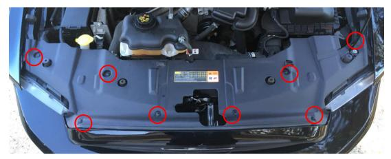
Step 2: Using a Philips head screwdriver and a ratchet with an 8mm socket, remove all the plastic and steel hardware which is holding the top of the bumper cover to the frame of the front end.
