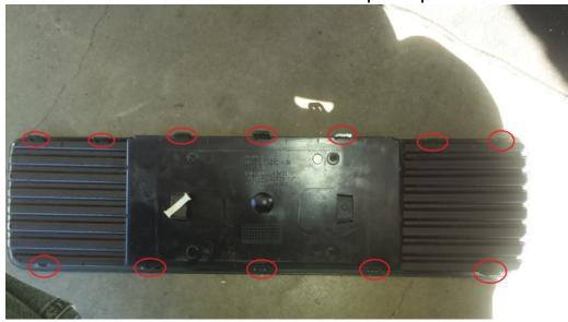
10. Install the carbon fiber license plate panel by inserting the tabs into the tab holes in the bumper cover. Then re-install the license plate light trim.
