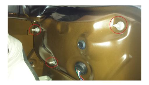
6. After the nuts are removed, hold the tail lens with one hand as the other hand pushes on the studs to un-mount the tail lens housing. Once the housing is a few inches away from the body reach behind the lens and disconnect the wiring harness by pressing on the gray tab on the side of the harness.
