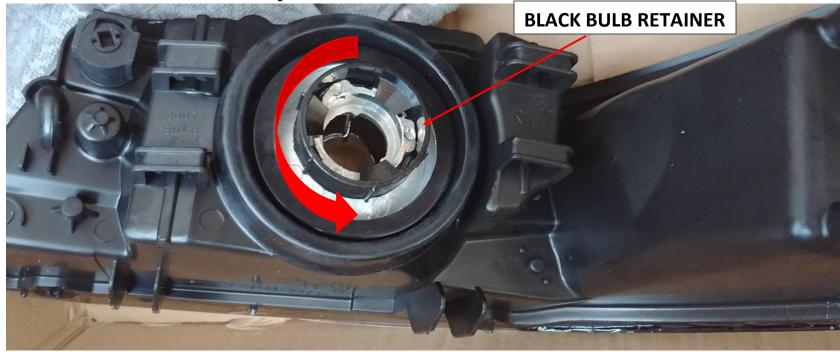
2. Twist off and remove black plastic bulb retainer
