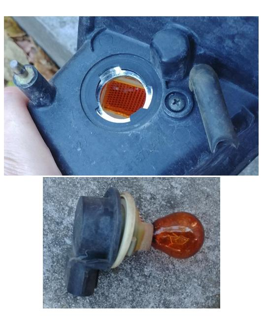
6. Twist and remove the grey plastic bulb retainer and then remove the headlight bulb and set both aside
