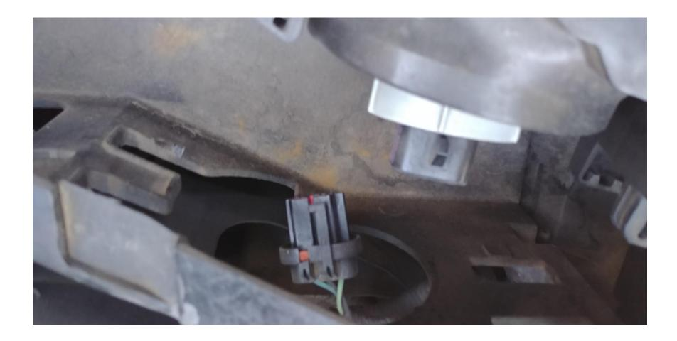
5. Twist 90 degrees and pull out side yellow light connector and set bulb aside
