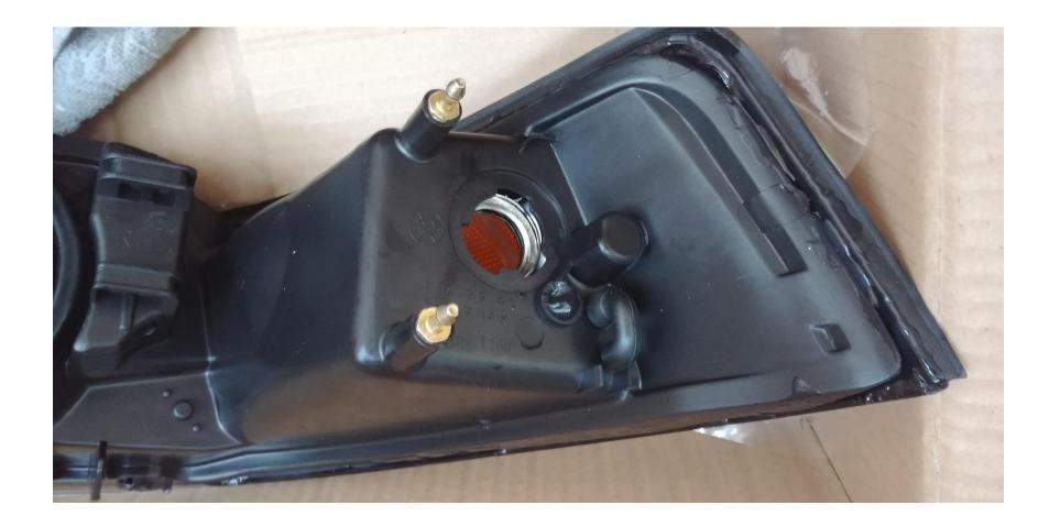
4. Insert the original bulb (or a new bulb) alighted with the internal tabs and place the black plastic bulb retainer on top of the bulb and twist it in to seal the bulb
