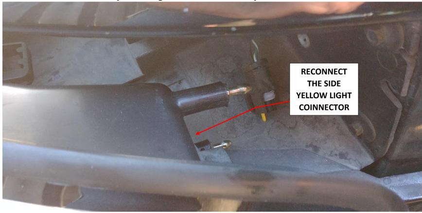
7. Reconnect the side yellow light connector to the yellow side bulb connector
