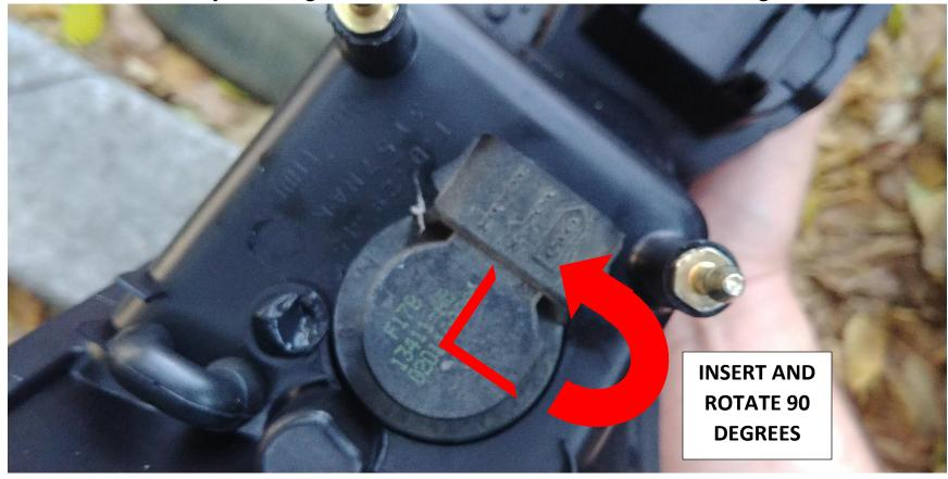
5. Insert the side yellow light connector into the hole and rotate 90 degrees
