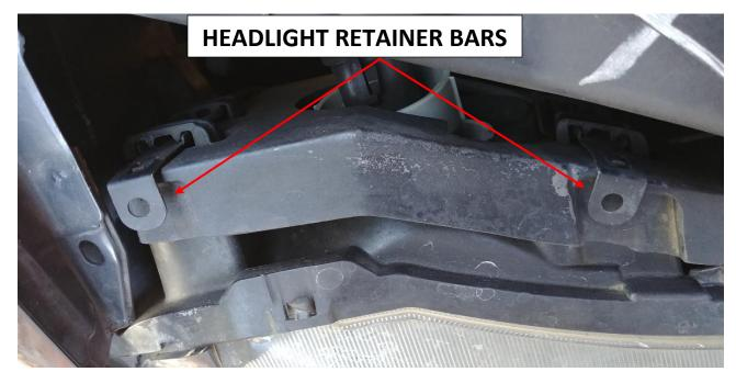
2. Pull the entire headlight slightly out of the body so that you can proceeded to disconnect the bulb connectors.
