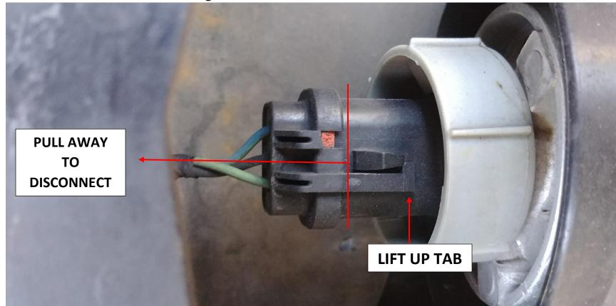
4. Disconnect front main headlight bulb connector
