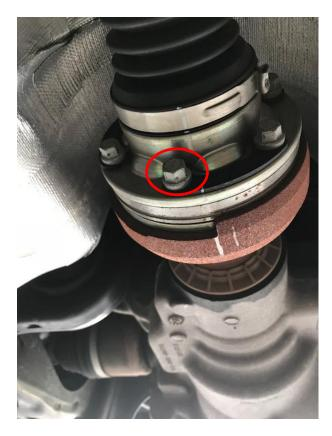
13. Remove 12mm driveshaft to transmission flange bolts located at front of driveshaft. (4 bolts in total)
