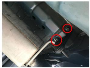
7. Exhaust hanger brackets have hooks attaching to vehicle. After bolts are removed the bracket must be lifted slightly to be unhooked.
