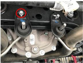
6. Remove 13mm bolts on muffler exhaust hangers. (4 bolts total)
