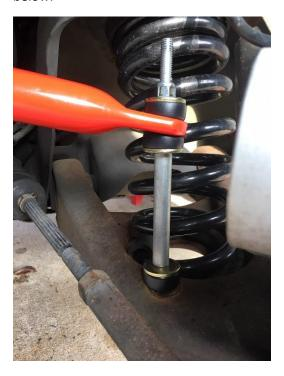
Step 14: Using your jack, slightly raise the control arm so that the bushings are resting in a completely horizontal position. You can now use the proper size socket to tighten the nut on top.
