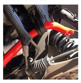
Step 10: With the new sway bar in place, but not yet tightened down, you will want to be certain that the sway bar is centered on the car. I used the marking provided by Eibach on the bar as the center point.
