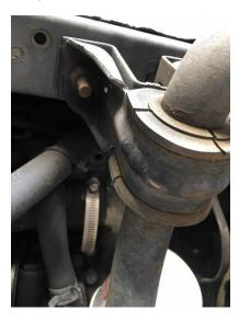
Step 6: With the brackets removed you can now lower the old sway bar out of the car.
