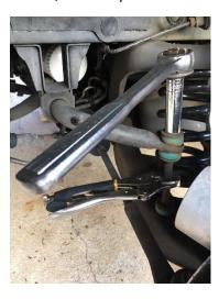
Step 3: With the nuts on both sides removed, you can now rotate the sway bar upwards. This will allow you to completely remove both end-links.
