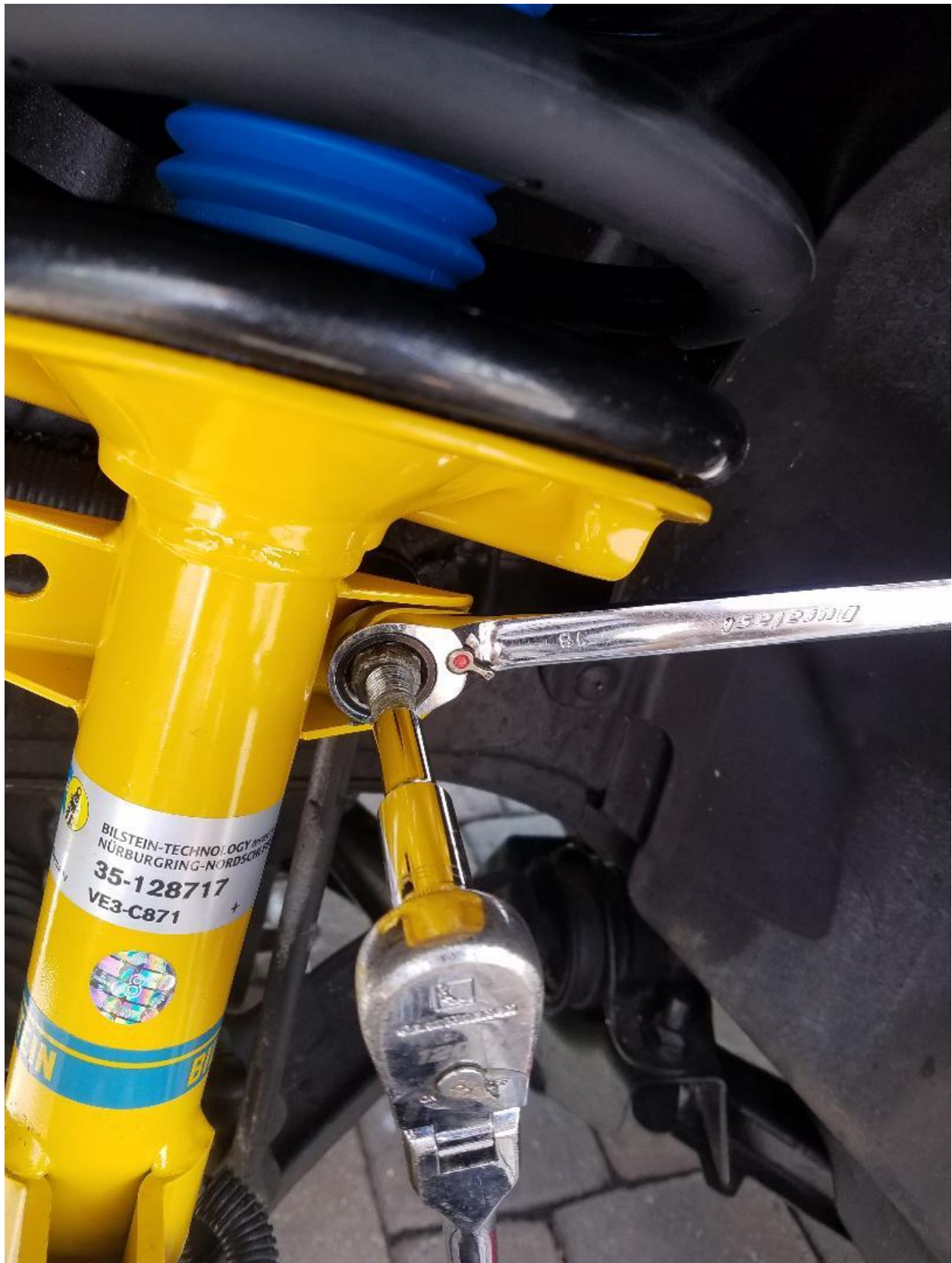
13. Reinstall the 10mm bolt for the brake hose/abs harness and tighten to 11 ft lbs
