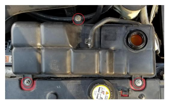
8. To install the new coolant reservoir slide it over the three holes where the bolts were removed earlier. Reinstall the three 11mm bolts and connect the two hoses into the same position. The clamps will need to be pinched again and slid into position at the end of the hose. The tank can now be refilled and reservoir cap reinstalled.
