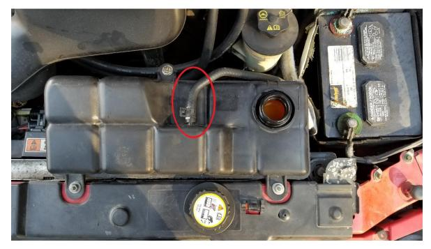
6. Now remove the second, larger hose located at the bottom driver's side of the coolant reservoir. A clamp will also need to be removed with a pair of pliers.
