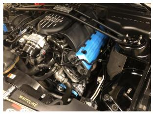
15. Reinstall all intake components (may very per application). Tighten all intake box bolts and metal clamps around the intake tube.
