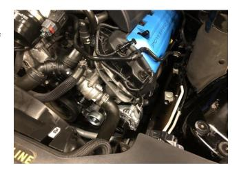
14. Position the new accessory belt loosely around the pulleys. Rotate the belt tensioner counterclockwise using a 15mm socket and a breaker bar. Slide the belt around the final pulley and slowly release the breaker bar to create tension on the belt.
