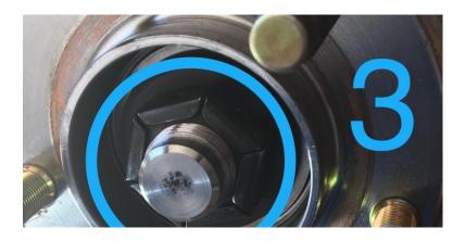
5) Remove spindle nut and the hub slides right off. set your old hub to the side so it can be compared to the new hub to make sure that the parts are compatible.
