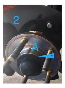
4) when the grease cap is removed the 36 mm nut will be exposed it is torqued at 221 pounds and loosens counterclockwise. The spindle nut that you take off is a one time use your new hubs from American muscle includes a new spindle nuts.
