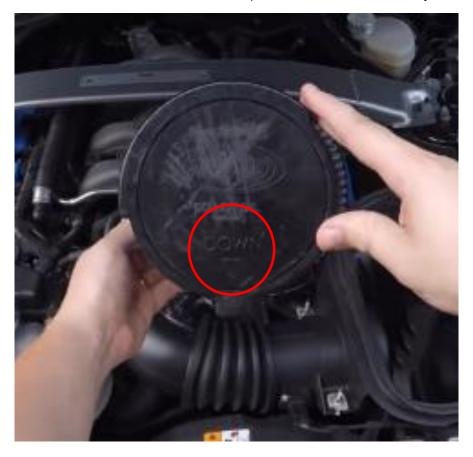
3. Ensure the band has the bolt head facing the front of the car for ease of tightening, you might have to flip it around if it was placed incorrectly at the
