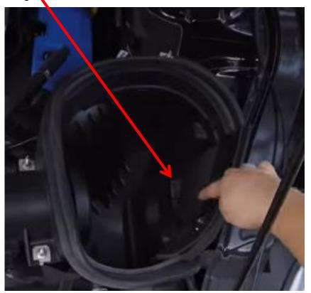
6. Use your 8mm socket to tighten the band snugly. There should be no play in the filter to keep the air intake pure.
