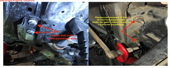
Step 6: Reach up and remove OEM bushings out from each side and replace with the new on. Place the 13mm bolts on each side of the bushing mount and hand tighten. You will not be able to replace the 15mm top bushing nut yet.
