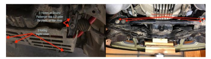
Step 3: Through the engine bay and using extensions socket remove the bushing nut (15mm) and the two frame bolts (13mm) on the sides of the bushing. (Long tube headers or other engine modifications may require you to access these by fully dropping the lower engine support)
