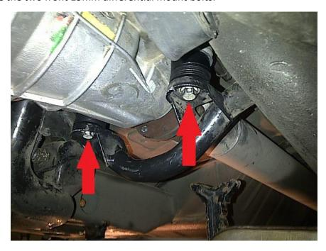
8. Loosen the two 21mm nuts holding the IRS crossmember (torque brace) to the subframe and slide it off the bolts.
