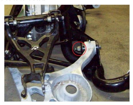
9. This should free up the differential enough to be remove the front differential bushings and any shimming washers. Pull apart each of the differential bushings and remove the m from the differential. For 03/04 Cobras remove the hanging NVH weight and bracket and leave it off. It will not fit correctly and is not needed with the upgraded front bushings.
