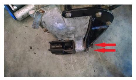
7. Remove the two front 15mm differential mount bolts.
