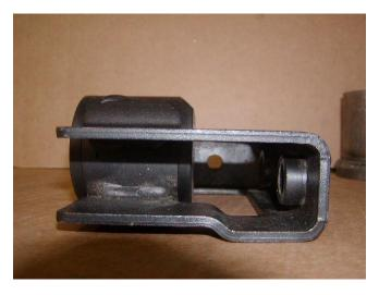
Note: The diff mount should be oriented with the bend on the top when installed
