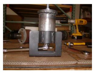
25. It is recommended to freeze the delrin bushings overnight to help them slide in easier. If extra force is needed, you may use a press if you have access to one like I did. Or if you flip the shell from in the bushing removal kit upside down and use a deep socket and extension, with the threaded rod/bolt and thick washer it can be used to slide the bushings in. The same can be done with the aluminum inner sleeve.
