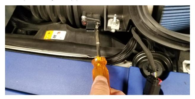
3. Replace MAF electrical connector. Be sure to push in the red locking tab.
