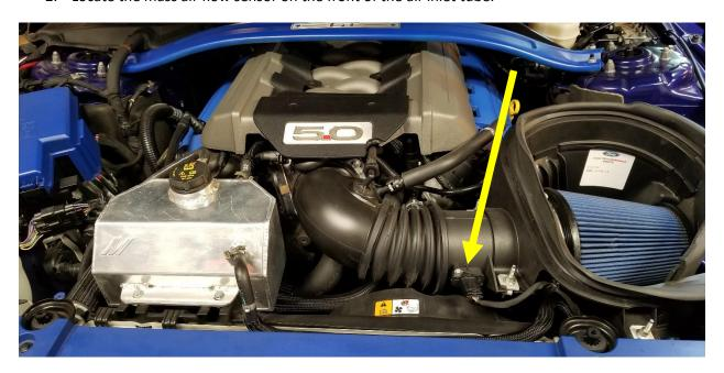
3. Disconnect the MAF connector by pulling back on the red tab and then pulling on the connector.
