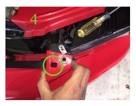
6) Before bumper removal use some painters tape on bumper and fender to safe guard paint while removing bumper. If you have an extra body it makes it easier to maneuver bumper removal pic 4 A
