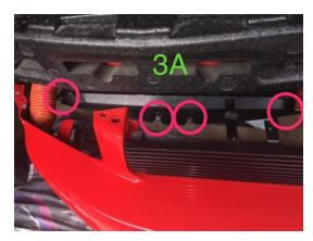
5 ) back on top remove the final push pins right hole from pillars in between headlights and grill lift the top upward to clear wedge hook then loosen to screws holding grill in place pic 4
