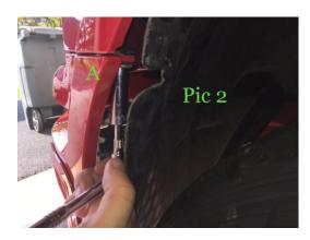
3) With hood up remove radiator service panel by sliding the center of 6 pushpin out with your flat blade screwdriver then slide the pushpin out set cover aside pic 3
