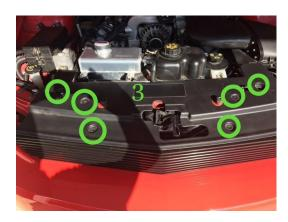
4) remove lower service panel with 5/16 socket to release the lower bumper cover Shown from top side after bumper is removed for a better visual location pic 3A
