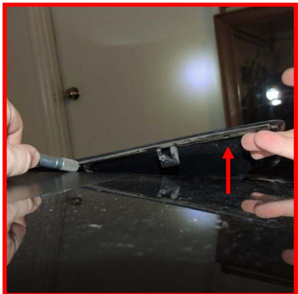
8. Continue to pull up on the driver side, carefully using the precision knife to cut the adhesive tape as you go. Again, stop before you reach the center stud (which had the nut on it from Step 4).
