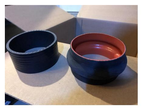
11. I chose to reuse the Paxton coupler as it allowed for a small amount of movement. This decision was based on the idea of having a small amount of angle movement at
