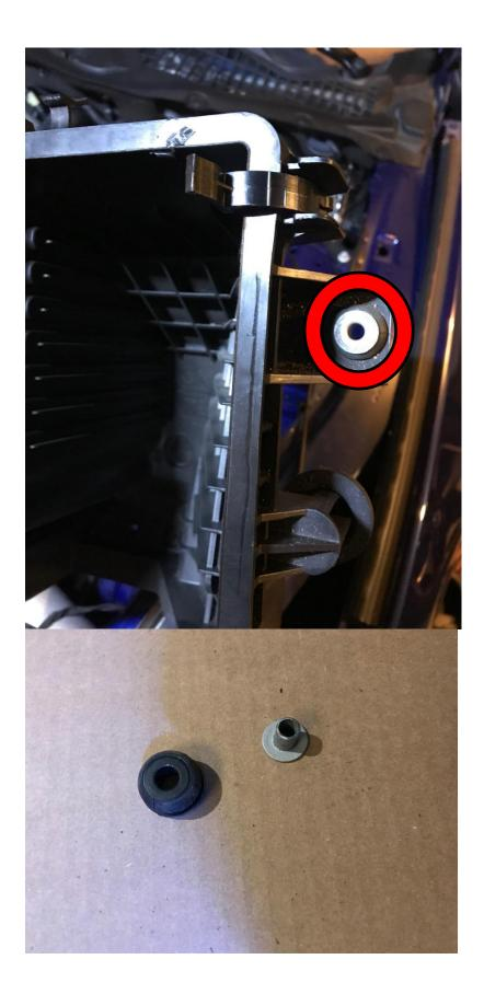
**8.** Install the insert and grommet in the JLT air box/shield in the same orientation as it was removed from the stock airbox.
