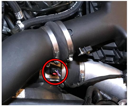
**2.** Loosen the 8mm bolts on the clamps securing the coupler between the air box and the blower inlet tube. Refer to image below.
