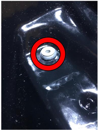
**9.** Place the JLT airbox/shield in the vehicle rotating it into place in a similar fashion as the stock airbox was removed. The front of the box/shield going in first and the rear rotating down into place. Check for clearance on surrounding components. Some trimming of the box/shield may be necessary to clear cold side piping coming from
