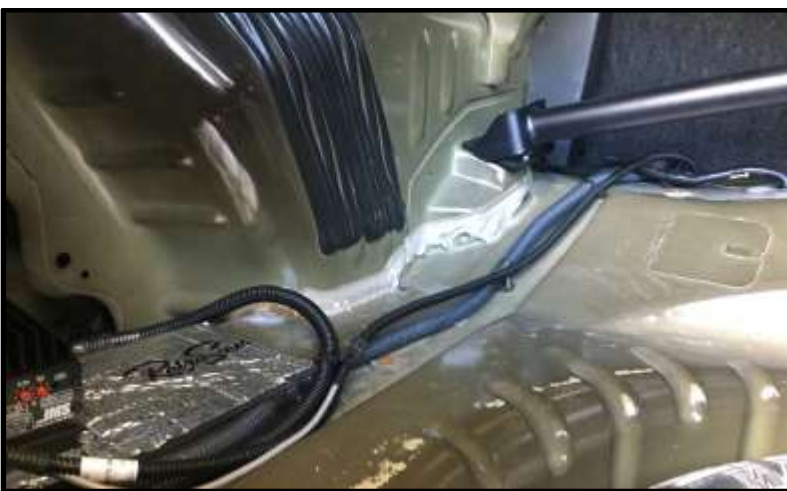
Figure F – Cable Routing from Trunk into Vehicle Cabin
