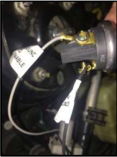
Figure N – Hobbs Switch Control Cable
