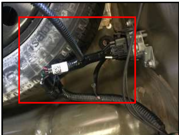
Figure E – JMS Plug & Play Fuel Pump Driver Module Harness (Spare tire left in for orientation)
