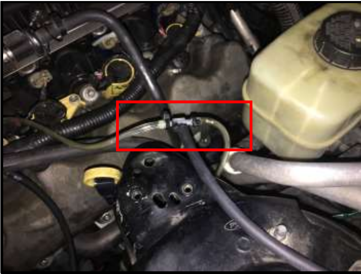
Figure L – Boost Source T-Fitting
