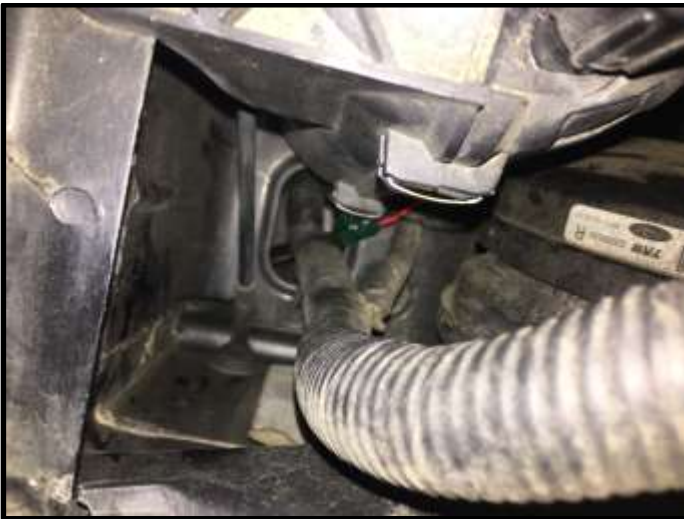
Figure K – Cable Routing Into Engine Compartment (Looking Down)
