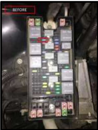
Figure O – Fuel Pump Fuse Replacement
