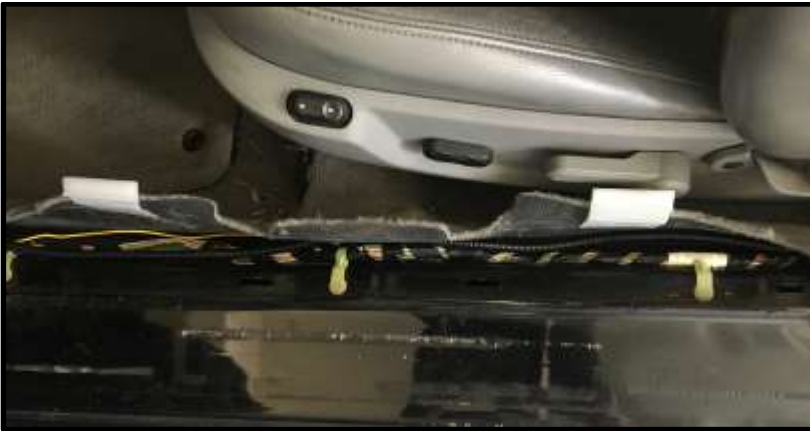
Figure H – Cable Routing Left of Driver's Seat
