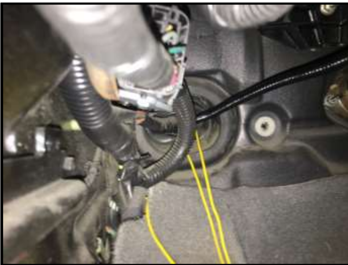
Figure I – Cable Routing Underneath Dashboard
