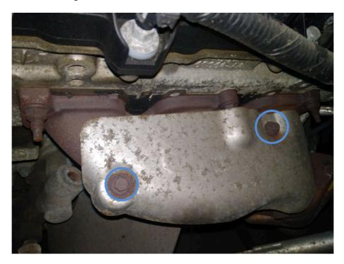
2. Unscrew 6 nuts using 13 mm socket/wrench. 3 of them are hiden under like on the patern below, to unscrew them use 3 inch extension.
