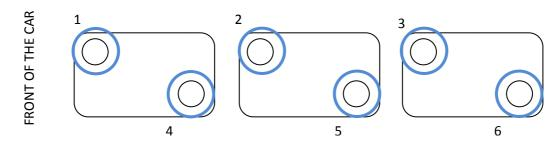
After removing the nut, remove the screws that are in engine block using 13 mm socket/wrench. Remove only 4 of them, number" 1; 2; 3; 5. Number 4 and 6 will help You with headers gasket and pre-assemble of the new MAC headers.
