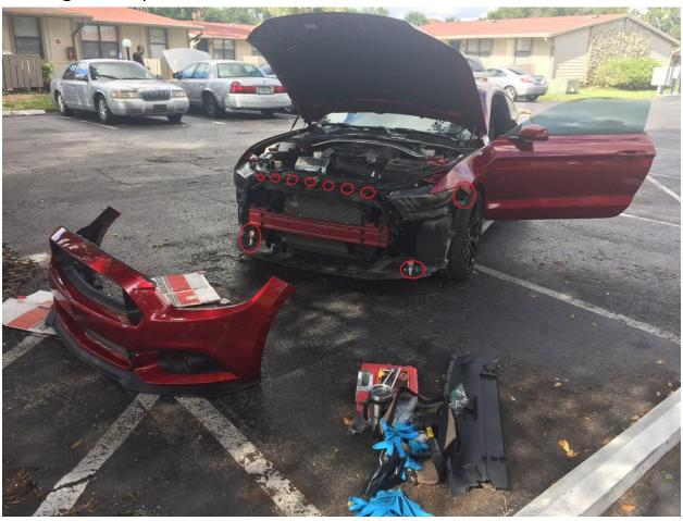
**Step 5:** Using a flat head screwdriver pry the tabs holding your grille to release it from the bumper. Be careful not to break the tabs
