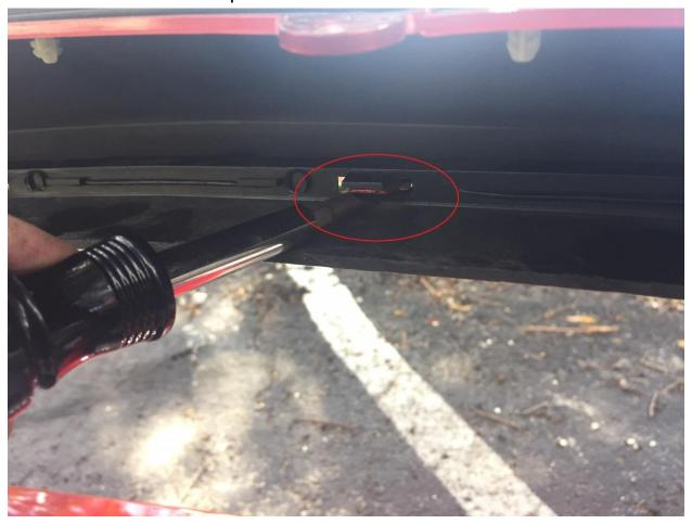
**Step 6:** Hold your new Modern Billet grille in place carefully lining up the spacing and mark your holes with a marker
