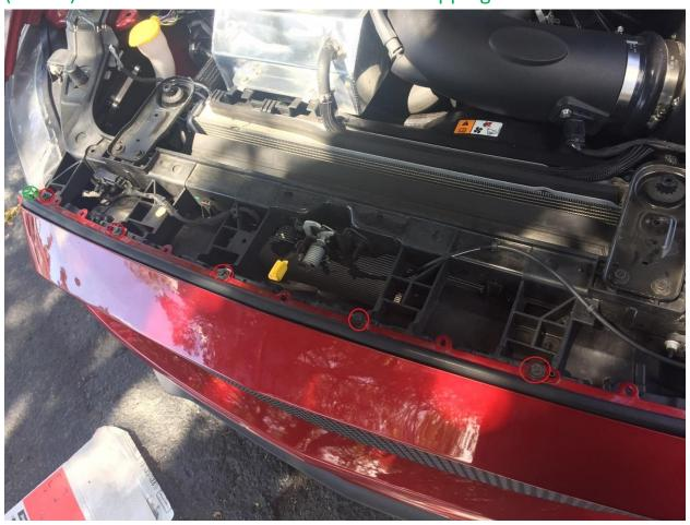
**Step 3:** Remove the screws holding your front splitter from underneath
