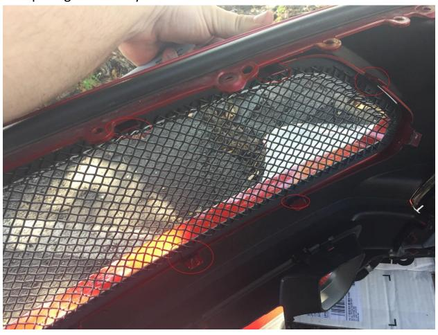
**Step 7:** Remove the grille and drill out the 14 holes marked with the marker. DO NOT attempt to drill through the grille tabs as it will cause your alignment to be off.
