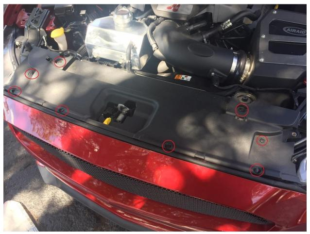
**Step 2:** Remove the screws holding your bumper on. (Red) 8mm (Green) 5.5mm hidden under the weather stripping on both sides
