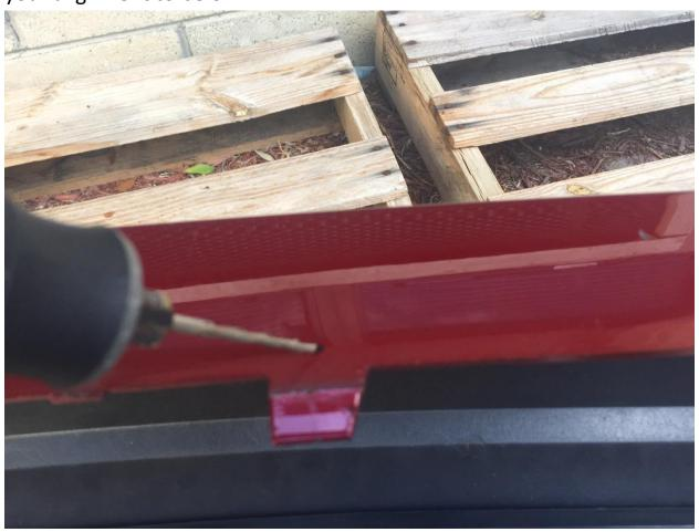
**Step 8:** Put your new grille back in the front bumper and secure the 14 screws and locknuts provided. Install all 14 loosely and slowly work your way around until all 14 are firmly secure
