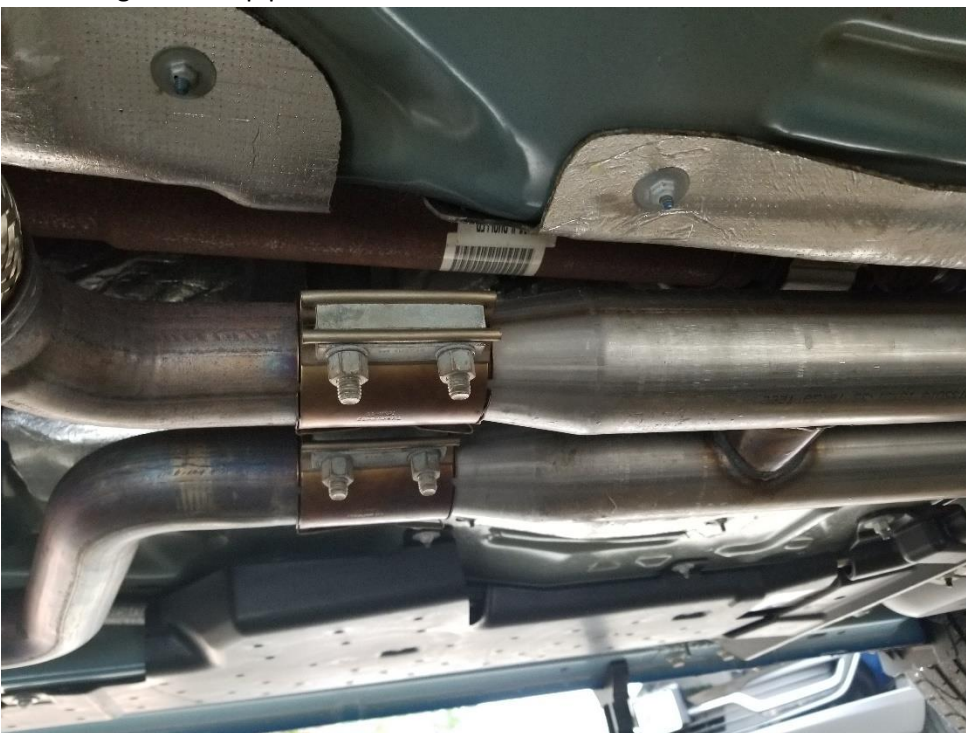
Figure 6 – H pipe installed on vehicle
