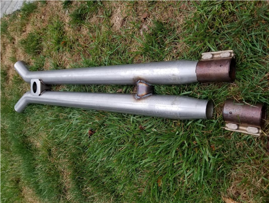
Figure 5 – how the clamps slide onto new H-pipe
