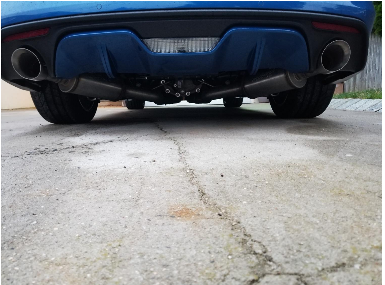
Figure 9 – exhaust fully installed
