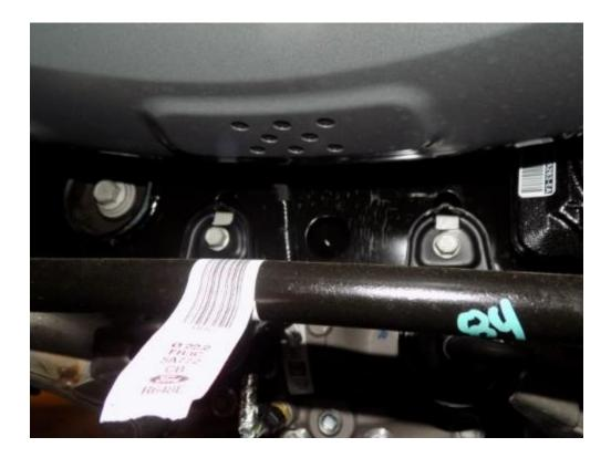
4. Loosen both clamps ahead of the resonator, lift the lock tabs and slide the clamps rearward to disconnect the OEM catback from the front section of the exhaust. Use caution, The OEM catback is one piece and heavy.
