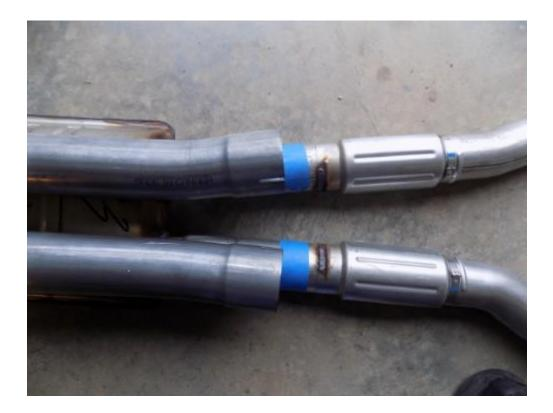
2. Measure 2" forward of the marks made in step 1 and scribe a cut line on the OEM pipes. The cut lines should be at the end of the straight section of pipe right next to the bends exiting the OEM Resonator. Using a Sawzall or similar tool, cut and deburr the OEM pipes with a file.
