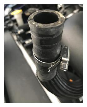
(Step 6) Remove the clamp from the bottom hose and slide on the new provided clamp. Tighten it just enough so it will not slide off.
