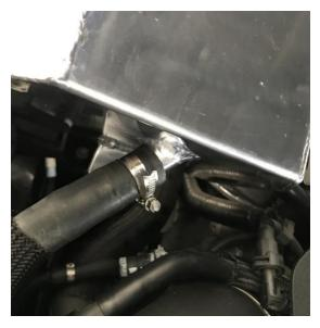
(Step 7) Install the hose to the bottom of the new tank then position and tighten the clamp.
