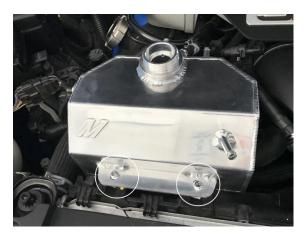
(Step 9) Line up the screw holes, install the new provided mounting bolts and tighten.
