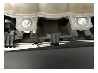
(Step 3) Remove the two existing mounting bolts from the factory tank.
