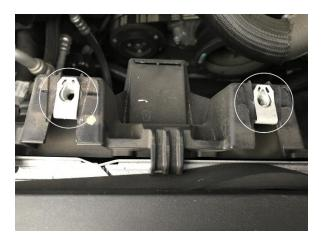
Be sure the existing mounting clips stay with the fan shroud.
