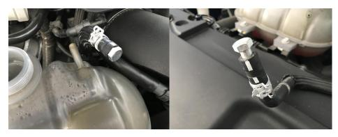
(Step 2) Cap off the hoses with a plug or bolt to prevent coolant leakage.
