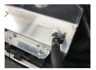
(Step 10) Remove the plug from one of the two top hoses and remove the factory clamp. Slide on the provided new clamp, install the hose to the new tank, then position and tighten the clamp.
