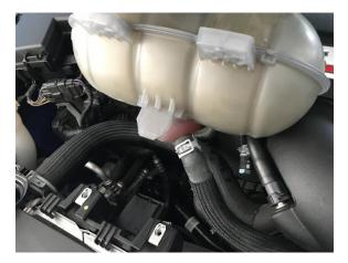
(Step 4) Lift the tank making sure the bottom hose stays connected. Empty the coolant from the factory tank into a small container (make sure it will hold all the coolant from inside the factory tank).
