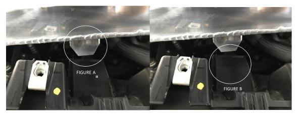
(Step 8) Place the cutout tab (Figure A) into the cutout slot (Figure B) on the fan shroud bracket.
