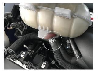
(Step 5) Remove the bottom hose, making sure it is kept upright so the coolant does not leak.
