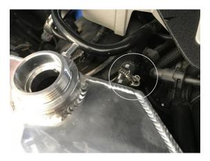
(Step 11) Repeat this step for the second top hose. Fill the new tank with the coolant drained from the factory tank and add additional coolant to the halfway point using the sight tube on the side of the tank if necessary. Install the factory cap on the new tank.
