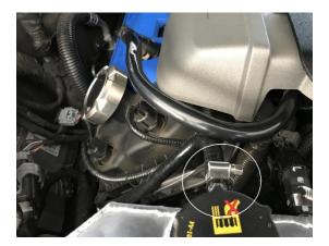
(Step 12) Install the provided vent tube with the provided clamp route it so it doesn't interfere with the fan or any other component.
