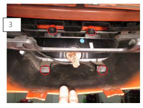
Disconnect the reverse light plug. Gently pull the bottom of the bumper down to access the (4) 7mm screws securing the 3rd brake light to the bumper. Remove the light from the vehicle. Reverse light and hardware will be reused.
