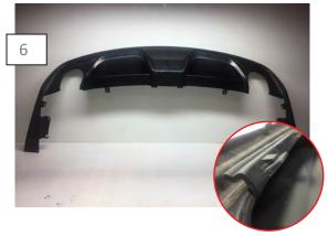
Install the Foose Diffuser on to the bumper trim. It will clip on the same as factory. Ensure the diffuser is fully clipped into the bumper trim before continuing.
