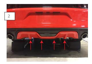
Remove the (2) push clips and (2) 7mm screws securing the factory diffuser to the vehicle.
