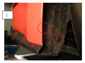
Support the rear of the vehicle so you can access the underside of the bumper. Remove (2) fender liner clips to gain access to the (3) 7mm bolt holding the rear bumper trim to the bumper. Remove these on both sides.
