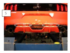
Once the factory trim panel is removed from the bumper, the factory diffuser will need to be cut from the bumper. Do this by cutting along the dotted lines shown above.
