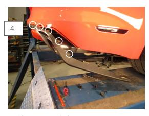
Apply firm pressure to the factory bumper trim to remove it from the bumper. The trim is clipped into the bumper.
