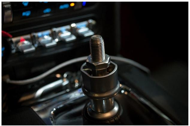
2. Once the existing shift knob is removed, install the retaining nut.
