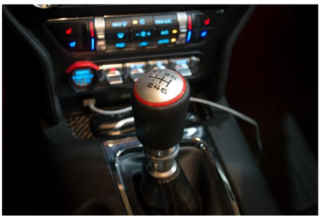
3. Install the GT350 Style Shift Knob. At this point, it may not line up correctly; if this is the case, remove the GT350 Style Shift Knob.
