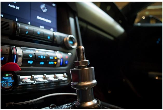
4. Loosen the retaining nut by turning it counter-clockwise. It took me roughly half a turn to align it correctly; however, individual mileage may vary and this may take several attempts.
